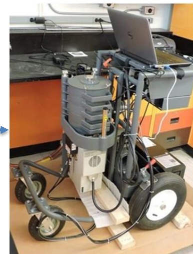
In-situ recording of the gamma-spectrum
