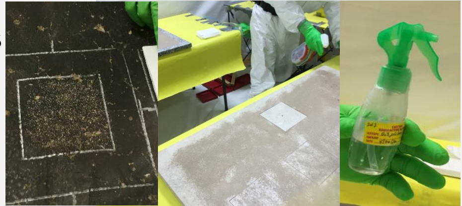
Application of particles and aqueous mist to surfaces
