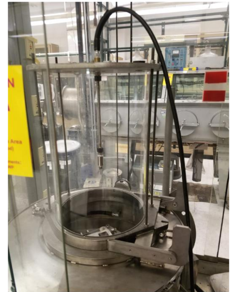
High pressure flow test chamber allows us to vary the spray pressure and coverage rates.
