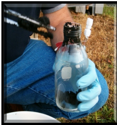
Collection of Biosolids Sample for Headspace Analysis of Volatile Organic Compounds
