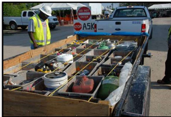
HHW Curbside Collection: Truck lined with bins to keep incompatible materials segregated.
