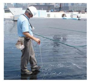
Photo 29.2 Example of flood electric field vector mapping Photo courtesy American Hydrotech, Inc
