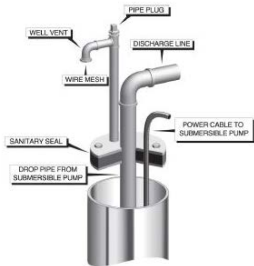
Figure 3-4: Submersible turbine upper well construction
