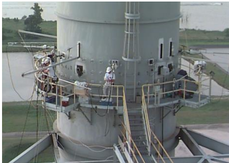
Stack testers performing a Relative Accuracy Test Audit. (EPA photo)
