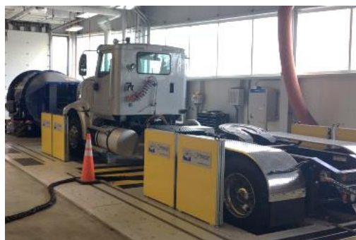
The back of a heavy-duty chassis dynamometer used for testing glider vehicles. (EPA OIG photo)
