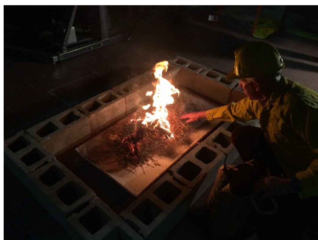
Left: Picture of fire emissions testing at Missoula Fire Sciences laboratory burn chamber (schematic at right)
