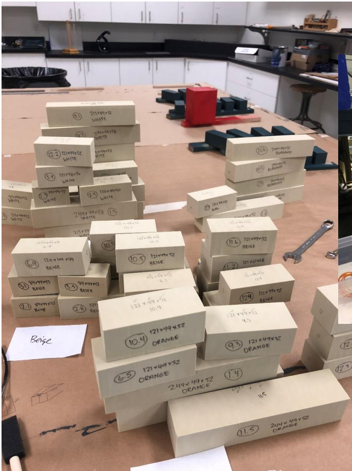
1:50-scale polyisocyanurate foam building structures
