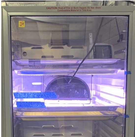
Aged in RH, UV controlled chamber
