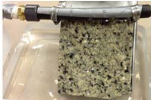
RAD decontamination testing of Wash Aid
