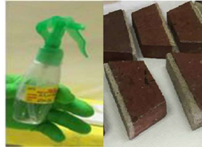
Application of contamination to the brick surfaces
