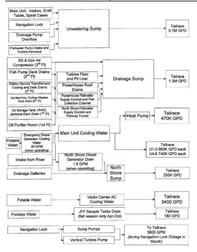
Lower Granite Lock and Dam and Process Diagram
