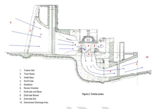
Figure 2. Cross-section of hydroelectric generating facility process
