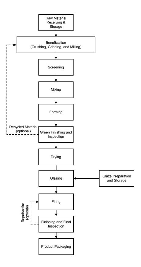
Figure 2-1. Ceramics Process Flow Diagram
