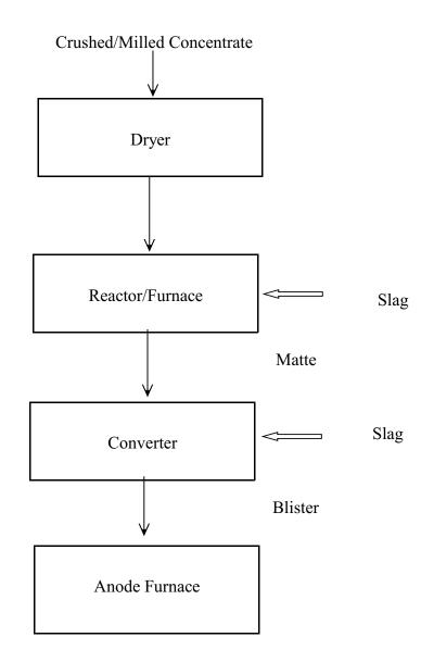
Figure 2-2. Flow Diagram of Primary Copper Smelting
