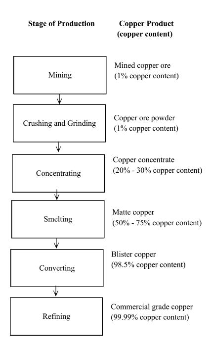
Figure 2-1. Flow Diagram of Primary Copper Production
