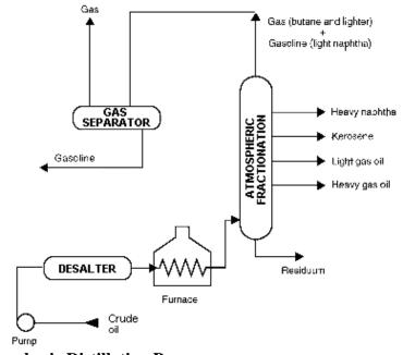
Figure 2-3 Atmospheric Distillation Process
