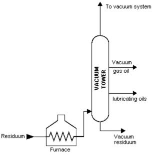
Figure 2-4 Vacuum Distillation Process
