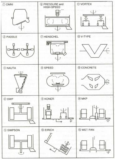
Figure 2-2. Mixing and Kneading Machines
