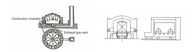
Figure 2-8. Round Kiln with Downdraft System
