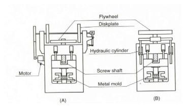
Figure 2-3. Vacuum Press (Friction, Hydraulic Press)
