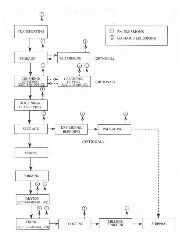
Figure 2-1a. Refractory Manufacturing Process Flow Diagram
