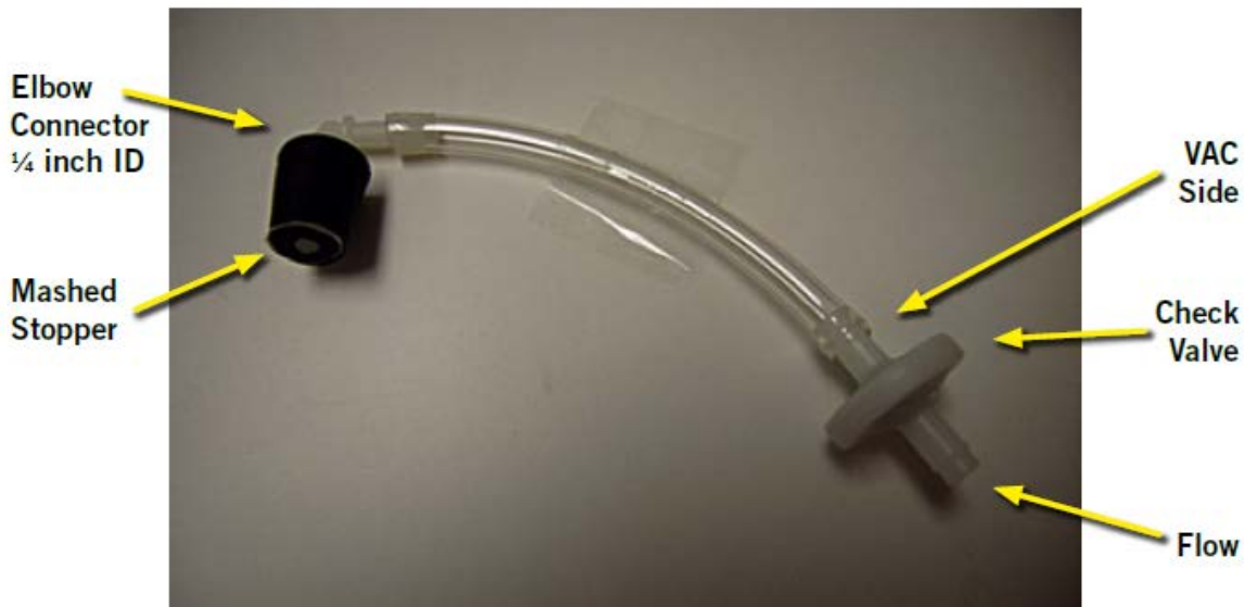
Figure 6 – Meshed stopper connected to check valve
