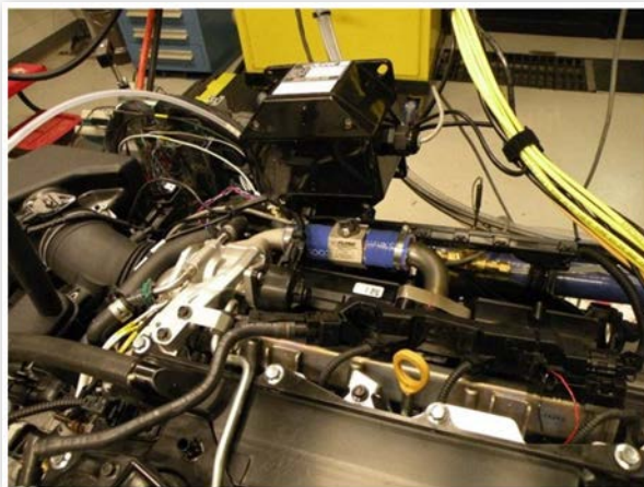
FIGURE 9 Fabricated/instrumented manifold with flow meter mounted on engine.
