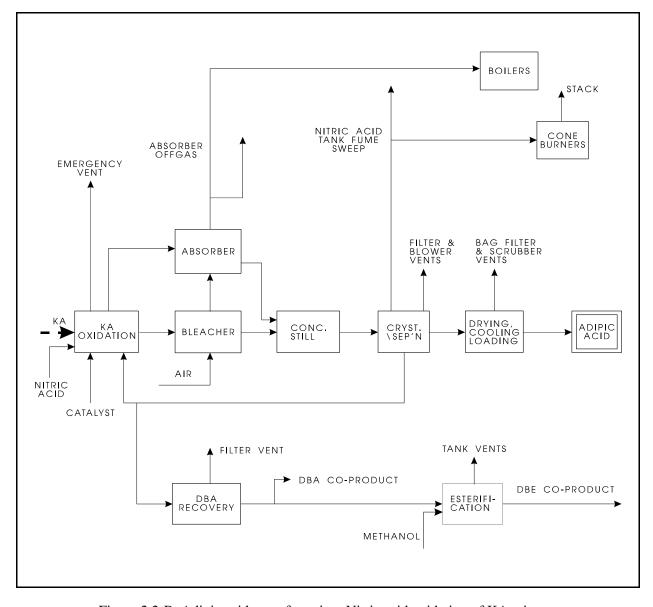
Figure 2.2-B Adipic acid manufacturing: Nitric acid oxidation of KA mixture
