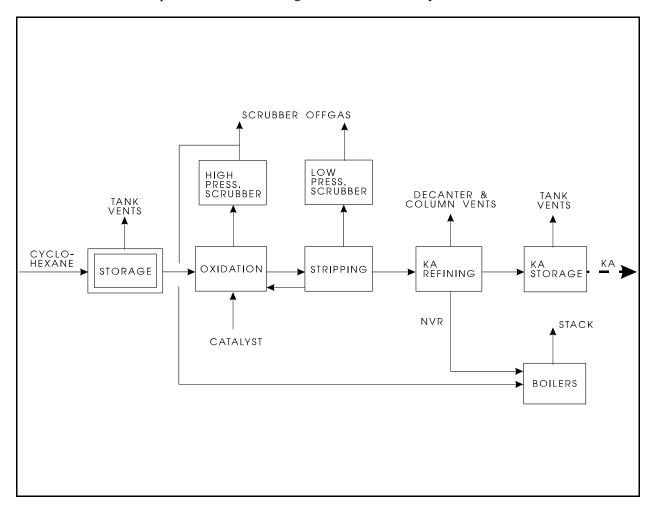
Figure 2.2-A Adipic acid manufacturing: Oxidation of cyclohexane
