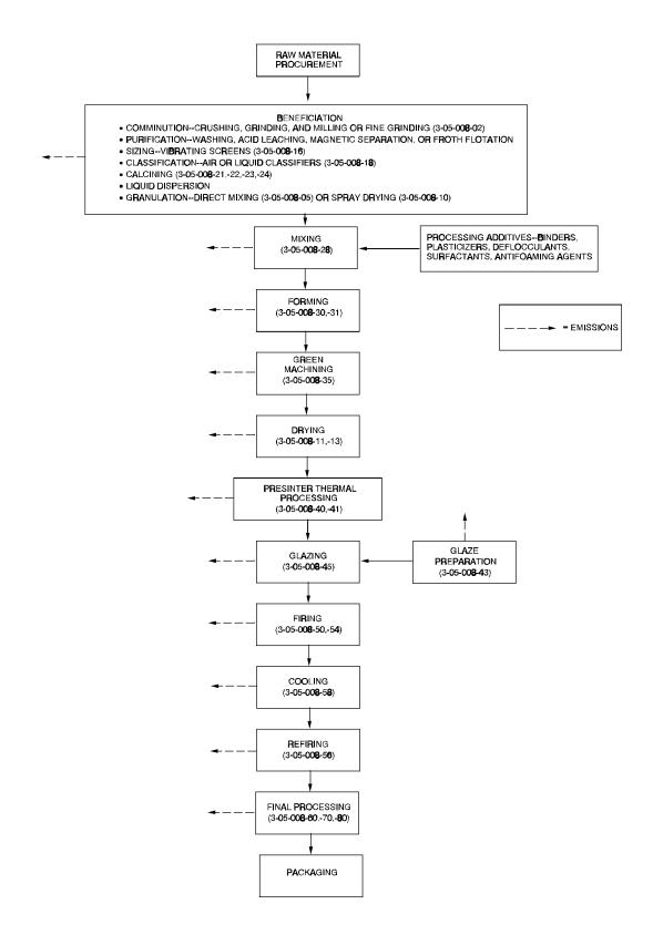
Figure 2-1. Process flow diagram for ceramic products manufacturing.
