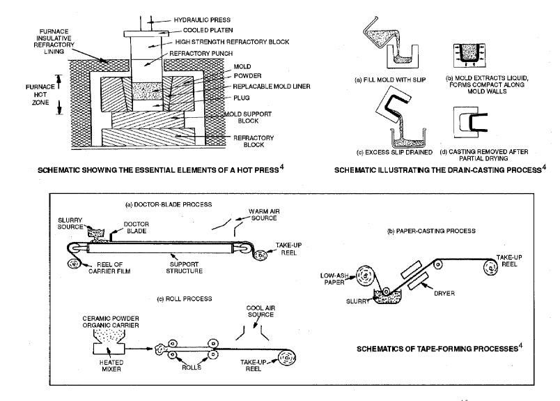
Figure 2-2. Miscellaneous ceramic products manufacturing processes and equipment.<sup>4,5</sup>
