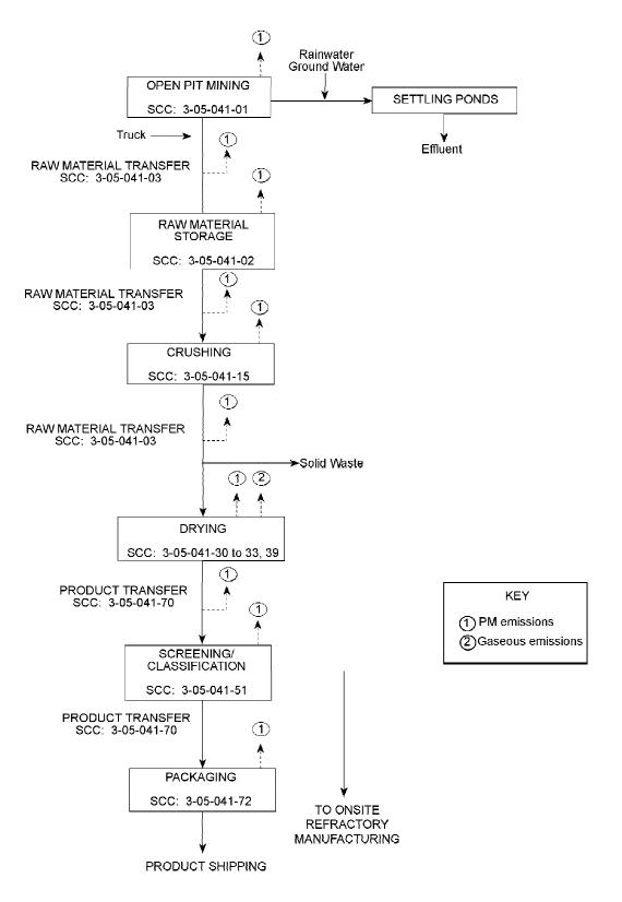
Figure 2-1. Process flow diagram for kaolin mining and dry processing. (SCC = Source Classification Code)
