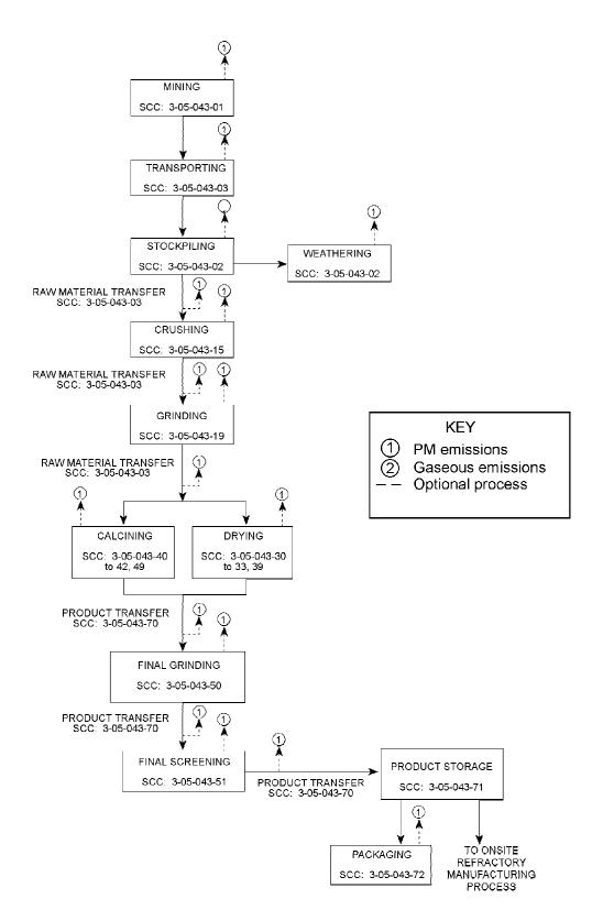
Figure 2-4. Process flow diagram for fire clay processing. (SCC = Source Classification Code)
