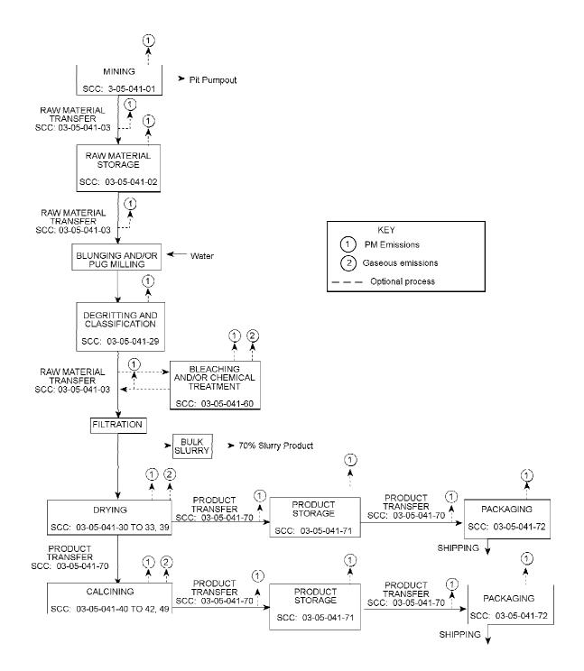
Figure 2-2. Process flow diagram for wet process kaolin for high grade products. (SCC = Source Classification Code)
