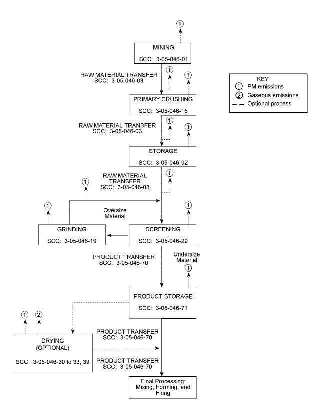
Figure 2-7. Process flow diagram for common clay and shale processing. (SCC = Source Classification Code)
