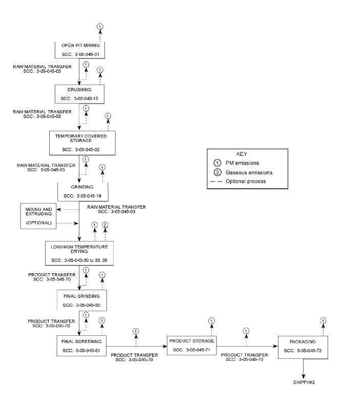
Figure 2-6. Process flow diagram for fuller's earth processing. (SCC = Source Classification Code)
