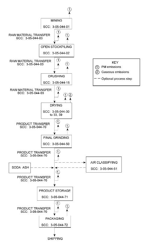
Figure 2-5. Process flow diagram for bentonite processing. (SCC = Source Classification Code)
