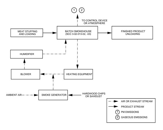
Figure 2-1. Typical batch smokehouse.<sup>1</sup>
