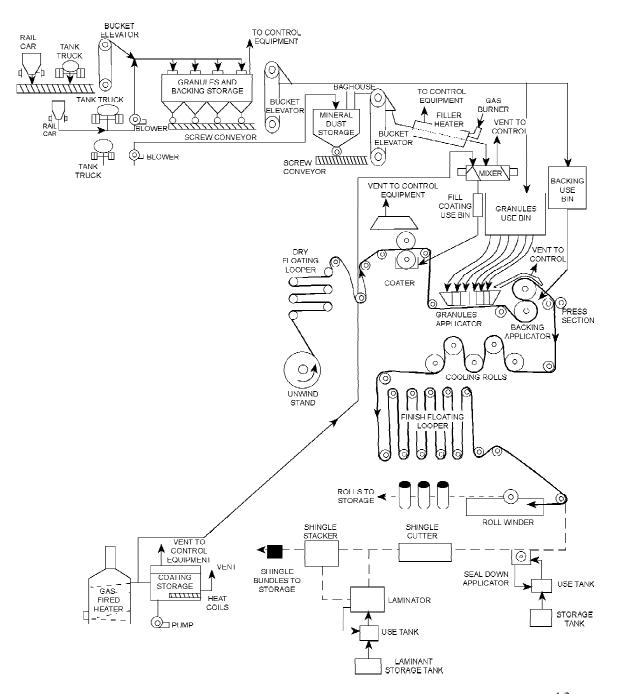
Figure 11.2-4. Fiberglass shingle and roll manufacturing process flow diagram.<sup>1,2</sup> (SCC = Source Classification Code)
