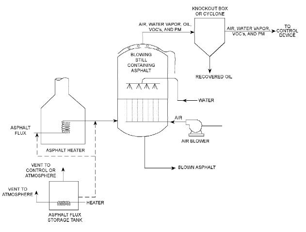
Figure 11.2-1. Asphalt blowing process flow diagram.<sup>1,4</sup> (SCC = Source Classification Code)
