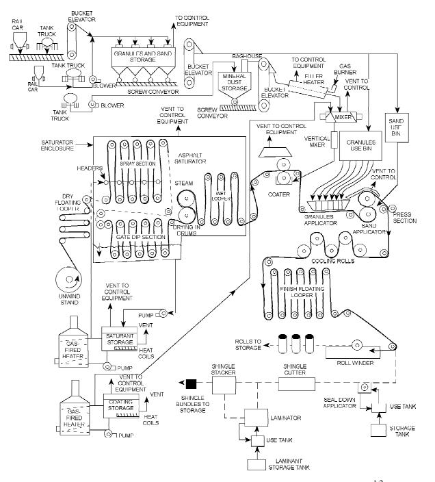
Figure 11.2-3. Organic shingle and roll manufacturing process flow diagram.<sup>1,2</sup> (SCC = Source Classification Code)
