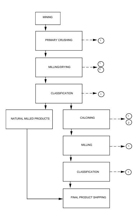
Figure 11.22-1. Typical process flow diagram for diatomite processing.
