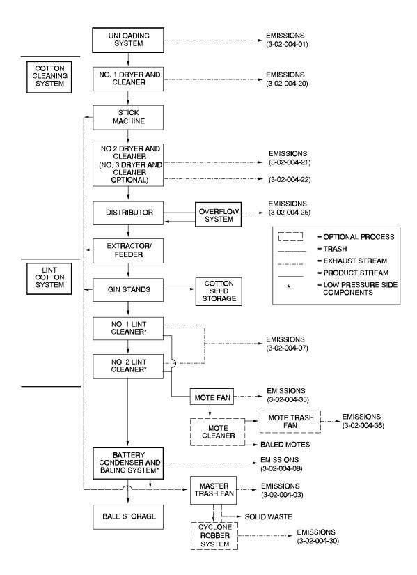
Figure 9.7-1. Flow diagram of cotton ginning process. (Source Classification Codes in parentheses.)
