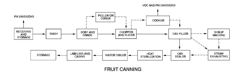
Figure 9.8.1-1. Generic process diagram for fruit canning.
