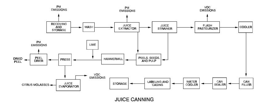
Figure 9.8.1-3. Generic process diagram for juice canning.
