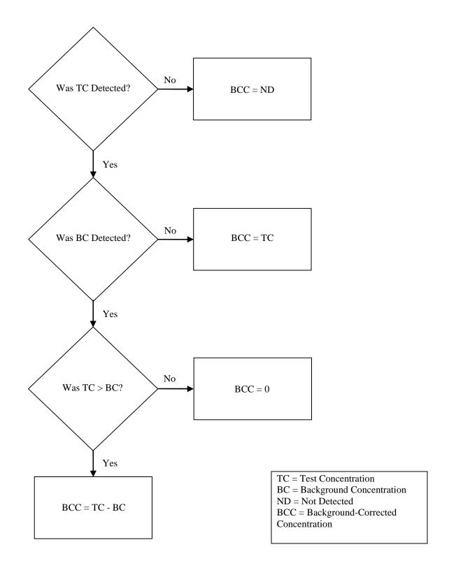
Figure 1 Calculation of background-corrected concentration.
