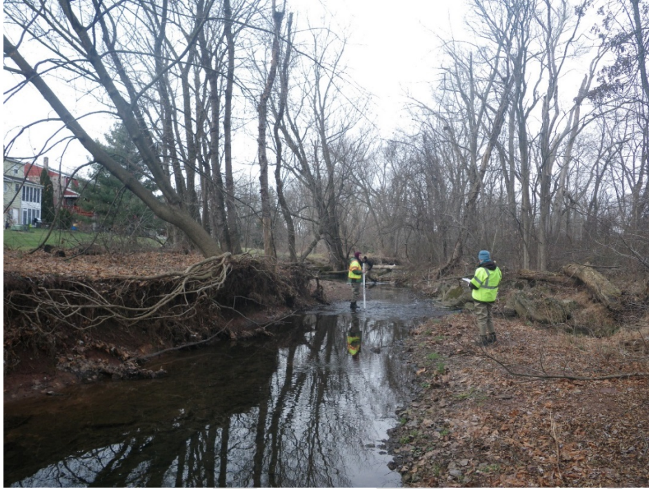
Figure E: Site 3, observable erosion on the left bank of the Indian Creek mainstem.
