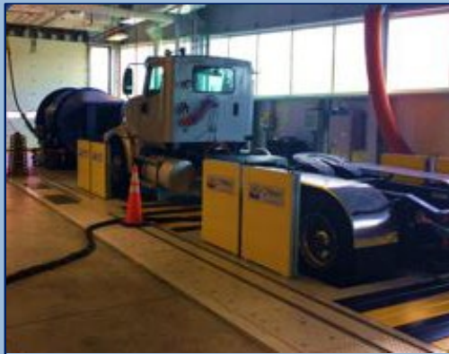
The EPA's heavy-duty chassis dynamometer. The top picture shows the front of the heavy-duty chassis dynamometer while the bottom picture shows the back. (EPA OIG photos)
