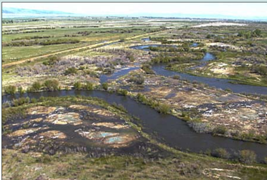
Overland runoff from exposed tailings and impacted soils, upper Clark Fork River, 1997.
