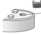
Replace access plug or install an inverted, screened well vent if one is not present. Silicone (or any other caulking) is not an acceptable permanent fix for any well opening deficiencies.
