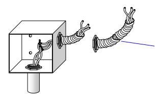
An electrical junction box shall be watertight (including at box attachment to the well casing and electrical conduits attached to the box) to prevent contaminants from entering the well. Replace damaged flexible conduit.
