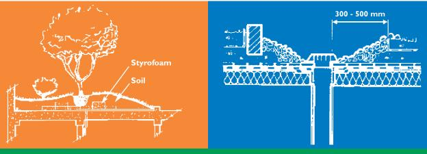
Fig. 8 – Deep Soil over Structural Column
