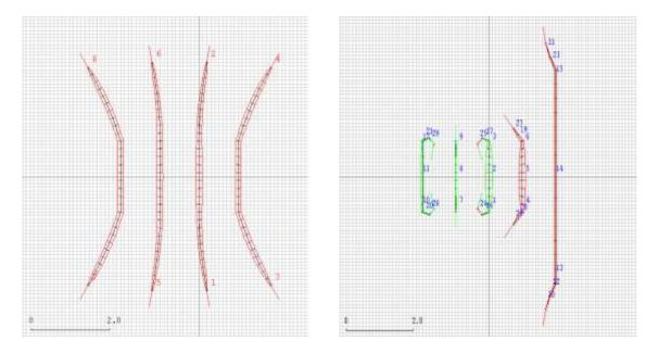
*Figure 5. Interaction of multiple fractures in a horizontal well. Green represents closed fractures. Note the fractures turning away from each other to follow the path of least resistance.*
