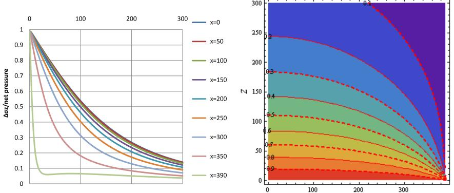
Analytical model for induced stress perpendicular to pennyrHF (stress shadow)-used for FRV
