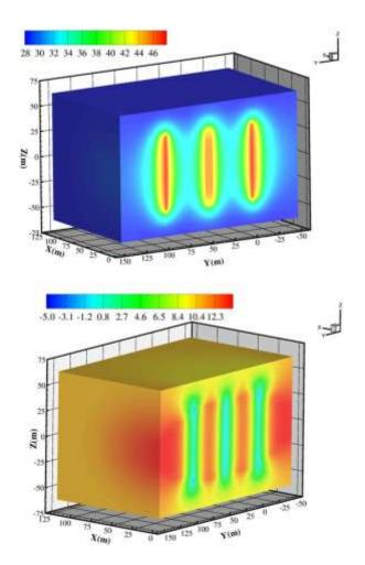
Figure 7. Distribution of pore pressures (MPa) in the formation; minimum principal effective stress (Barnett shale,  $0.09 \text{ m}^3$ /s per fracture; 3 hrs) (Rawal & Ghassemi, 2011).
