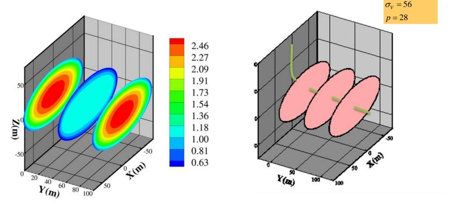
Fracture aperture distribution (in cm) after 3 hours of pumping.
