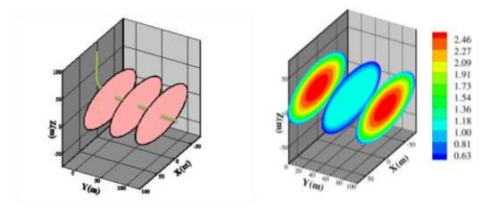
Figure 6. Fracture aperture distribution (in cm) after 3 hours of pumping in Barnett shale.
