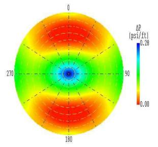
Figure 3. Structural Permeability Diagram for New Albany Shale ( $\mu$ =0.6).
