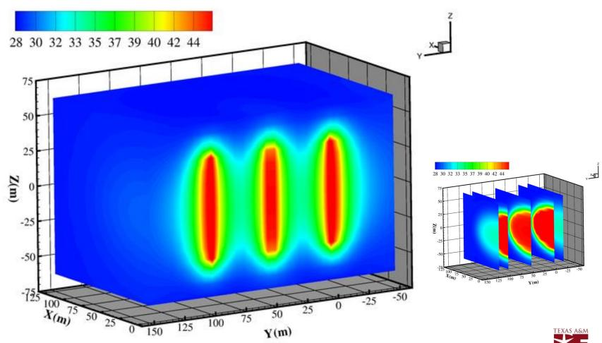
Distribution of pore pressures (MPa) in the formation after 3 hrs of injection
