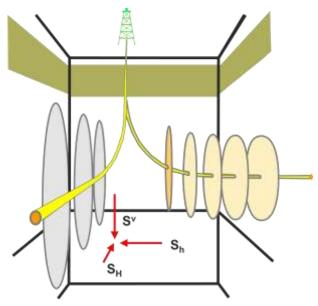
Figure 4. Fracture orientation in horizontal wells.
