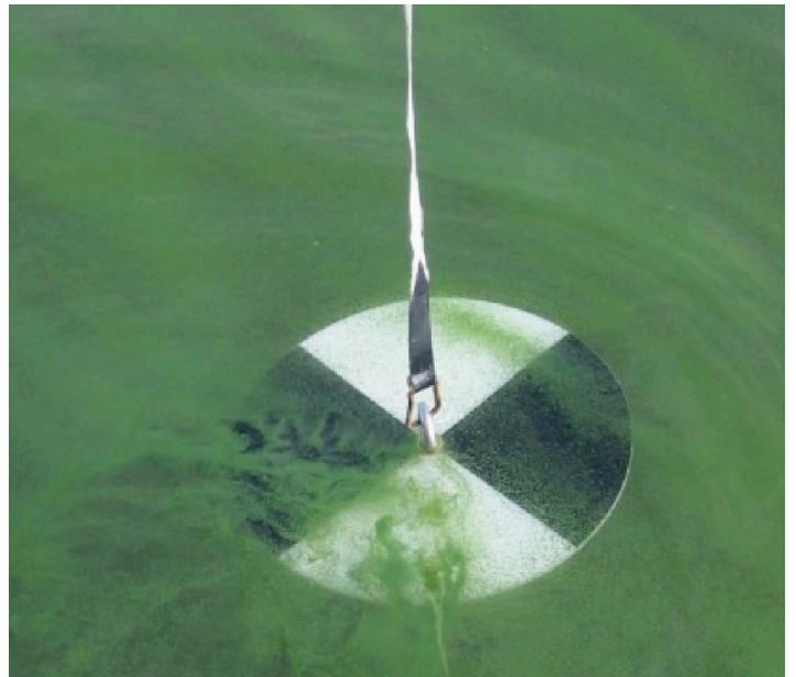
Figure 4. Secchi disk measuring the Secchi depth in water with extensive algal growth. Credit: Photo courtesy of USGS
