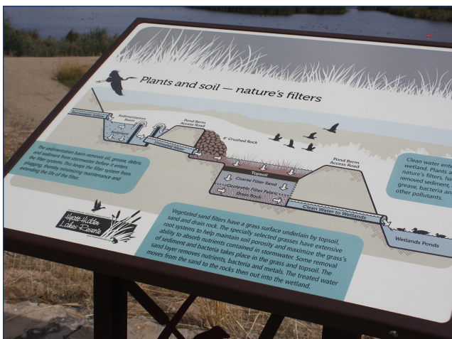
Image 7: Sand filter components. (Photo courtesy of Kris Wagoner)
