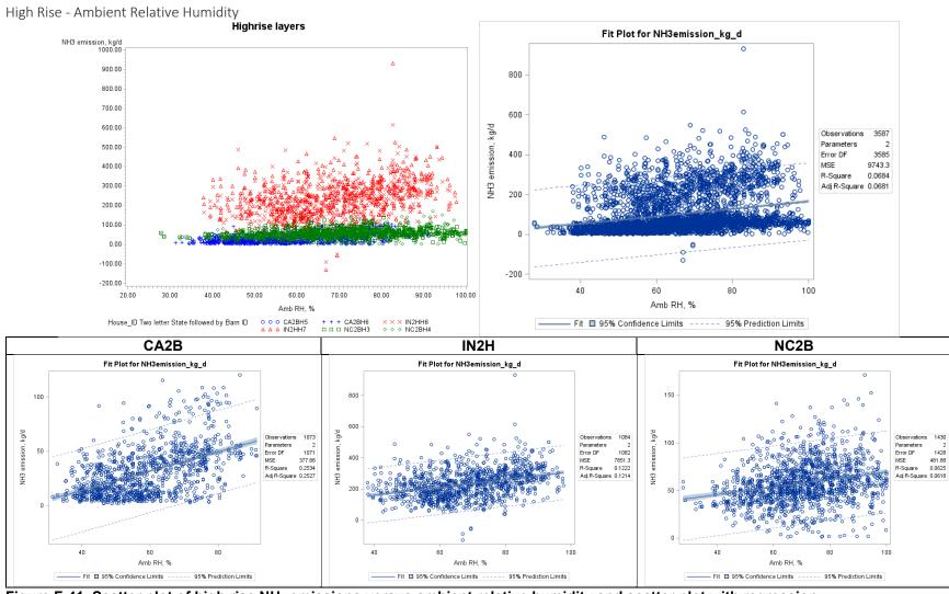
Figure F-41. Scatter plot of high rise NH<sub>3</sub> emissions versus ambient relative humidity and scatter plot with regression.
