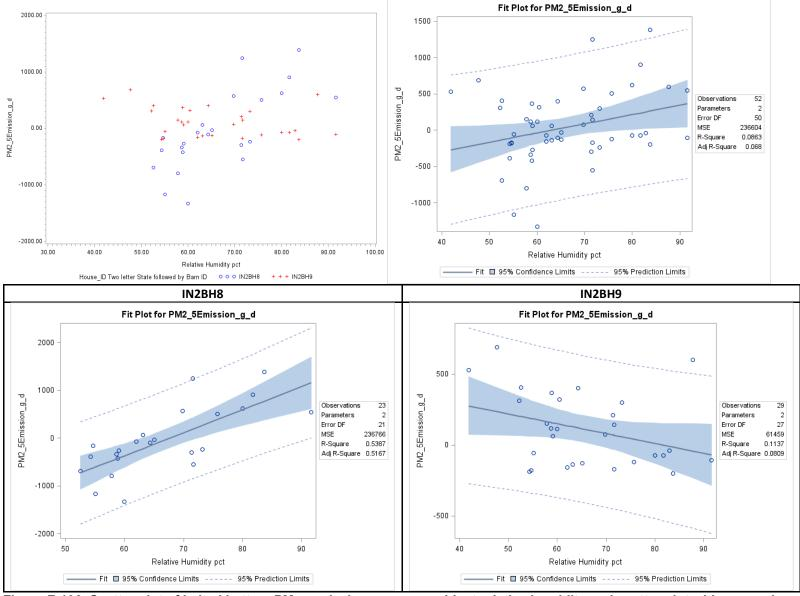
Figure F-106. Scatter plot of belted battery PM<sub>2.5</sub> emissions versus ambient relative humidity and scatter plot with regression.
