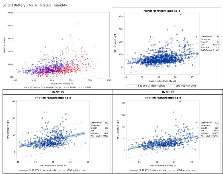
Figure F-88. Scatter plot of belted battery NH<sub>3</sub> emissions versus house relative humidity and scatter plot with regression.
