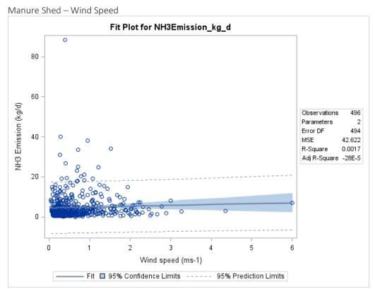
Figure F-155. Scatter plot of manure shed NH<sub>3</sub> emissions versus wind speed and scatter plot with regression.
