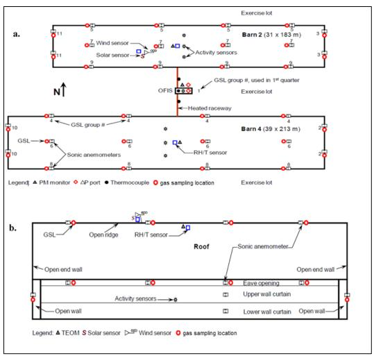
Figure 8-21. Overhead (a.) and side (b.) view of sensor measurements at WA5A barn (Ramirez-Dorronsoro et al. 2010).
