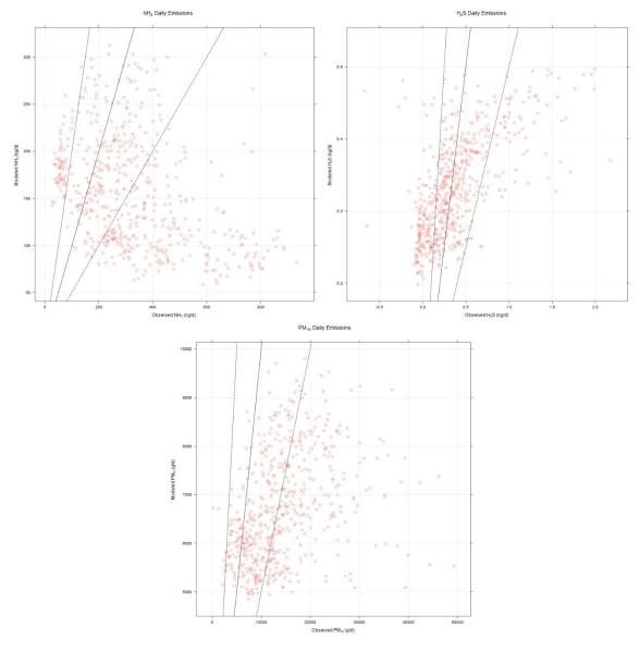
Figure H-4. Scatter plots of model versus observed emissions.
