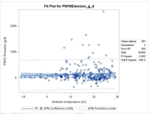
Figure F-147. Scatter plot of manure shed  $PM_{10}$  emissions versus ambient temperature and scatter plot with regression.
