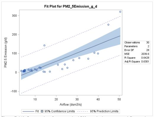
Figure F-143. Scatter plot of manure shed PM<sub>2.5</sub> emissions versus airflow and scatter plot with regression.
