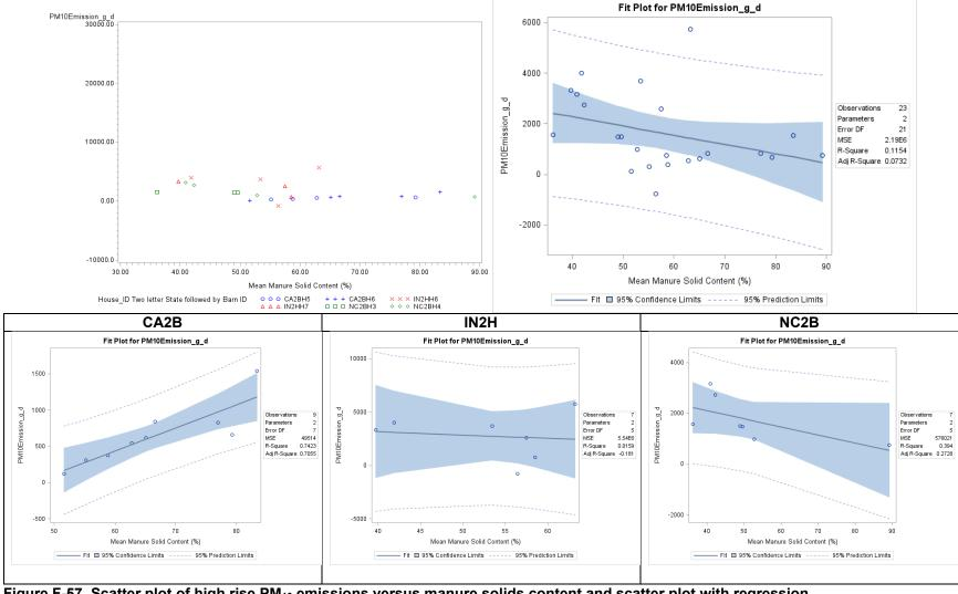
Figure F-57. Scatter plot of high rise PM<sub>10</sub> emissions versus manure solids content and scatter plot with regression.
