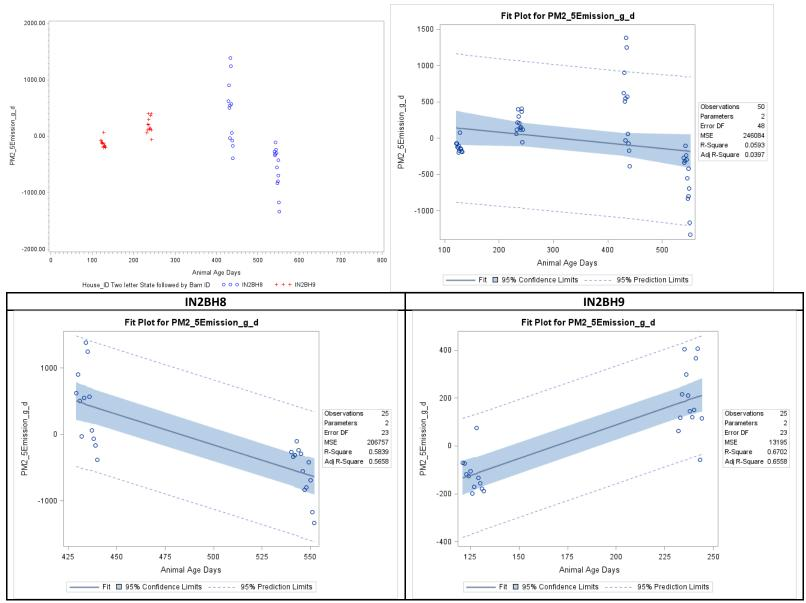
Figure F-81. Scatter plot of belted battery PM<sub>2.5</sub> emissions versus hen age and scatter plot with regression.
