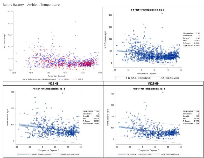
Figure F-98. Scatter plot of belted battery NH<sub>3</sub> emissions versus ambient temperature and scatter plot with regression.
