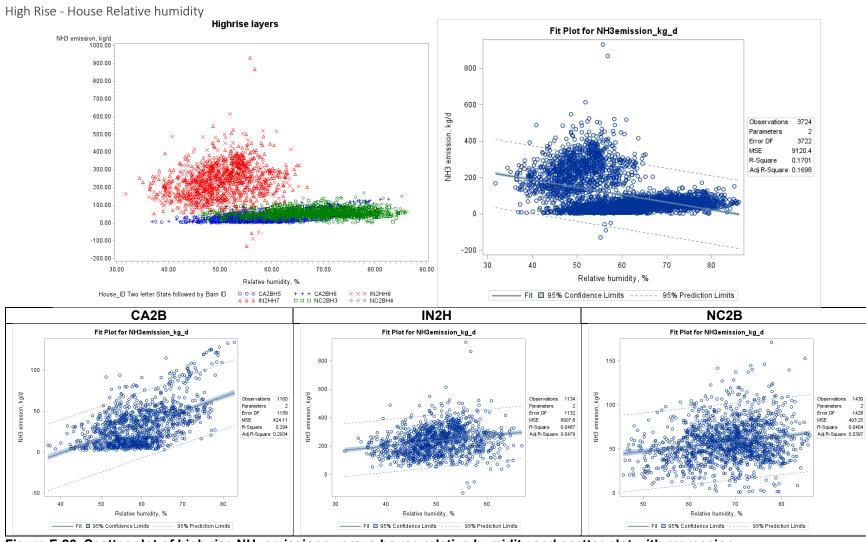
Figure F-26. Scatter plot of high rise NH<sub>3</sub> emissions versus house relative humidity and scatter plot with regression.
