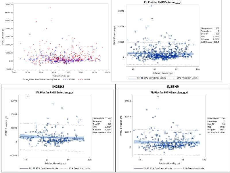
Figure F-105. Scatter plot of belted battery PM<sub>10</sub> emissions versus ambient relative humidity and scatter plot with regression.
