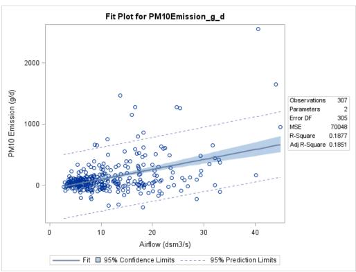
Figure F-142. Scatter plot of manure shed PM<sub>10</sub> emissions versus airflow and scatter plot with regression.
