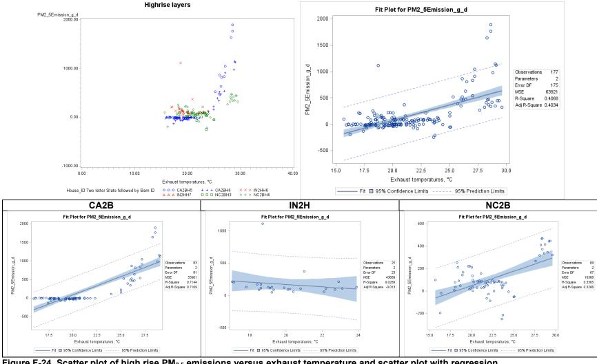
Figure F-24. Scatter plot of high rise PM<sub>2.5</sub> emissions versus exhaust temperature and scatter plot with regression.
