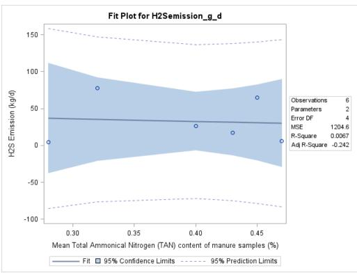
Figure F-172. Scatter plot of manure shed  $H_2S$  emissions versus TAN and scatter plot with regression.
