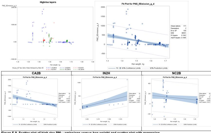
Figure F-9. Scatter plot of high rise PM<sub>2.5</sub> emissions versus hen weight and scatter plot with regression.
