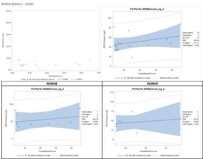
Figure F-112. Scatter plot of belted battery NH<sub>3</sub> emissions versus manure solids content and scatter plot with regression.
