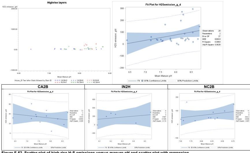
Figure F-52. Scatter plot of high rise H₂S emissions versus manure pH and scatter plot with regression.
