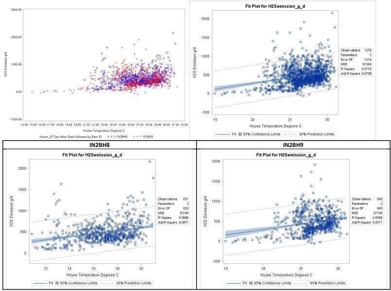
Figure F-84. Scatter plot of belted battery H<sub>2</sub>S emissions versus exhaust temperature and scatter plot with regression.
