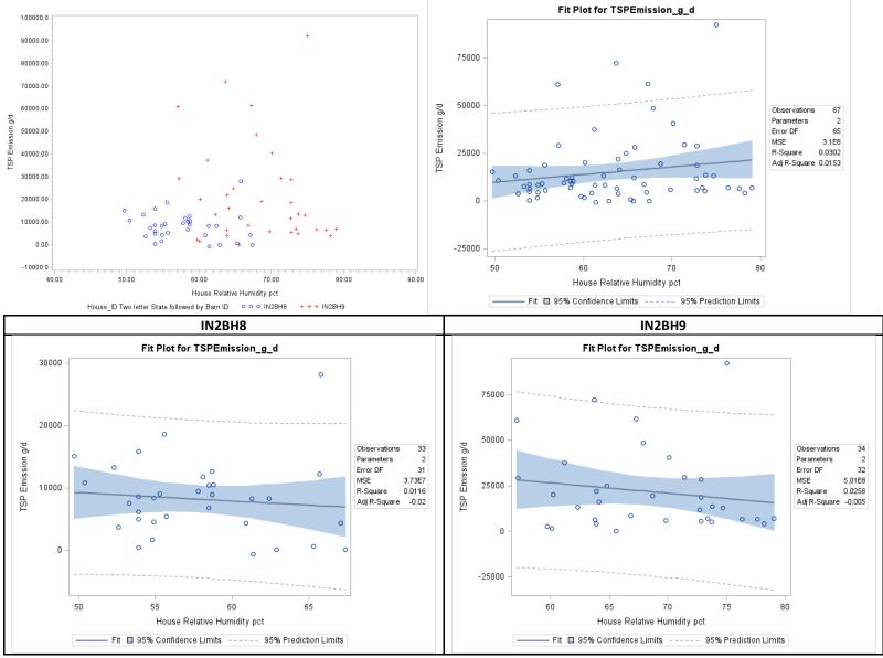
Figure F-92. Scatter plot of belted battery TSP emissions versus house relative humidity and scatter plot with regression.
