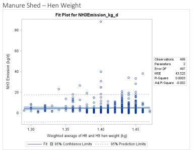
Figure F-125. Scatter plot of manure shed NH<sub>3</sub> emissions versus hen weight and scatter plot with regression.
