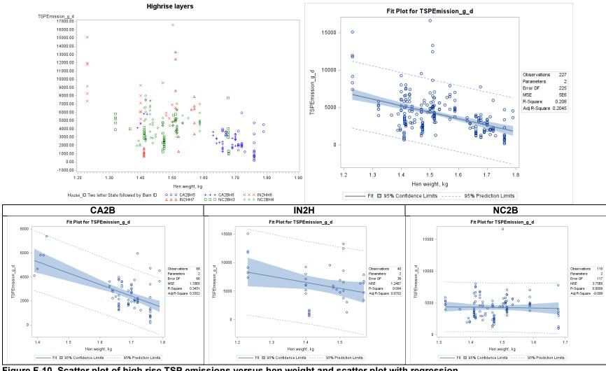
Figure F-10. Scatter plot of high rise TSP emissions versus hen weight and scatter plot with regression.
