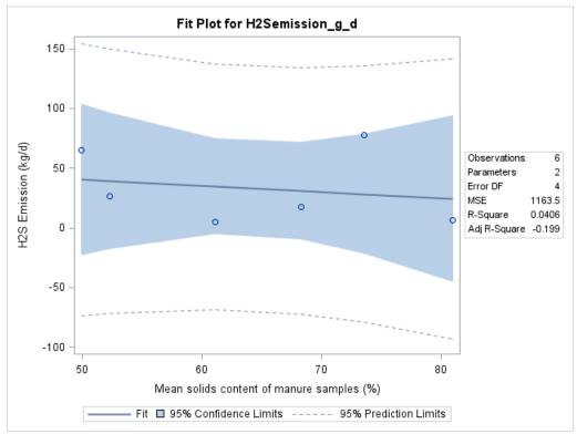
Figure F-169. Scatter plot of manure shed H<sub>2</sub>S emissions versus manure solids content and scatter plot with regression.
