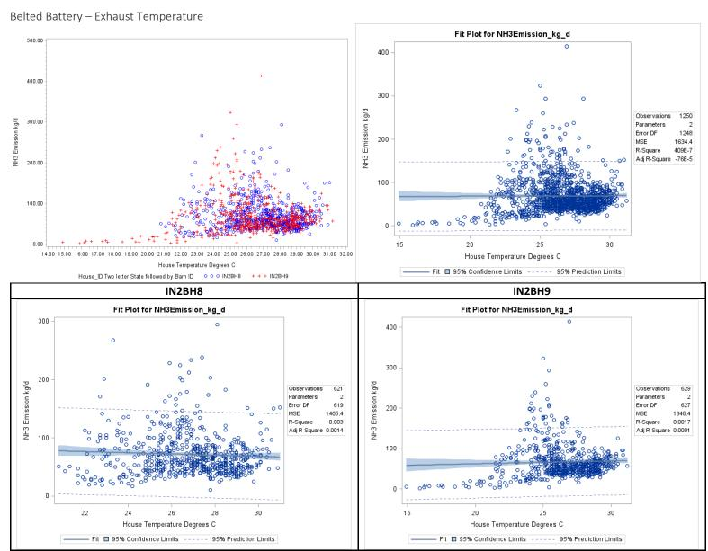
Figure F-83. Scatter plot of belted battery NH<sub>3</sub> emissions versus exhaust temperature and scatter plot with regression.
