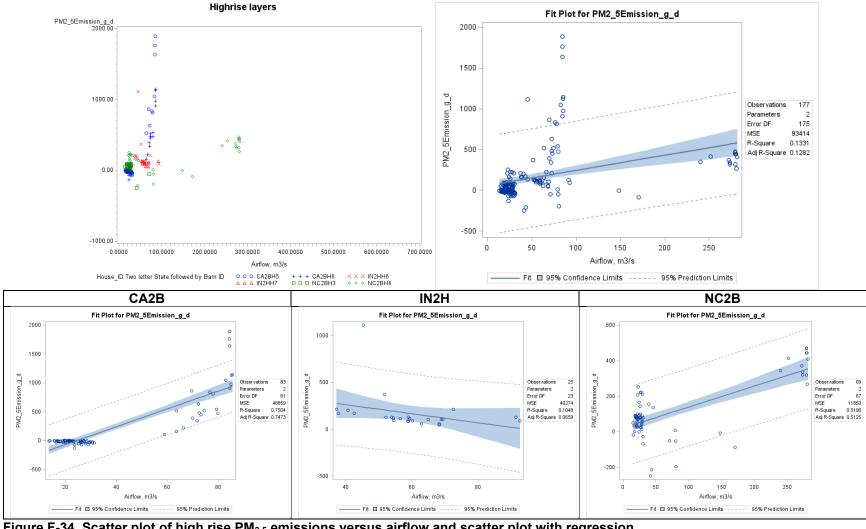
Figure F-34. Scatter plot of high rise PM<sub>2.5</sub> emissions versus airflow and scatter plot with regression.
