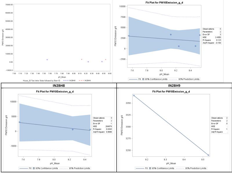
Figure F-110. Scatter plot of belted battery PM<sub>10</sub> emissions versus manure pH and scatter plot with regression.
