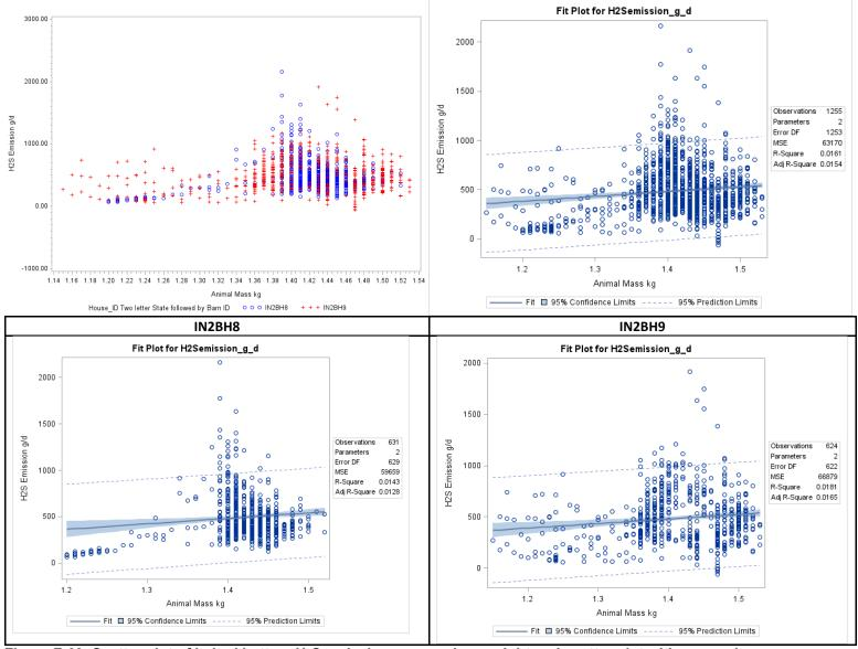
Figure F-69. Scatter plot of belted battery H<sub>2</sub>S emissions versus hen weight and scatter plot with regression.
