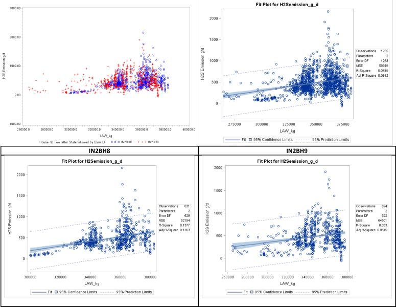
Figure F-74. Scatter plot of belted battery H<sub>2</sub>S emissions versus live animal weight and scatter plot with regression.
