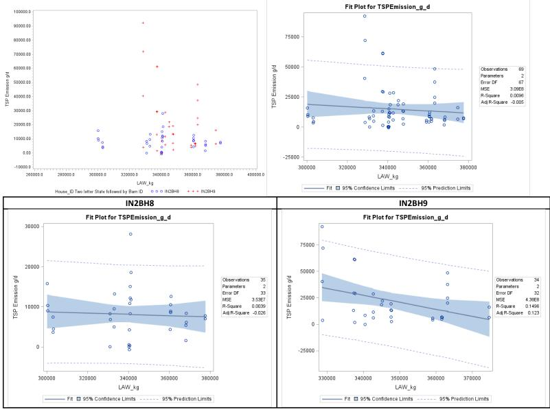
Figure F-77. Scatter plot of belted battery TSP emissions versus live animal weight and scatter plot with regression.
