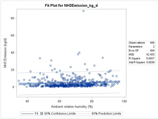
Figure F-150. Scatter plot of manure shed NH<sub>3</sub> emissions versus ambient relative humidity and scatter plot with regression.
