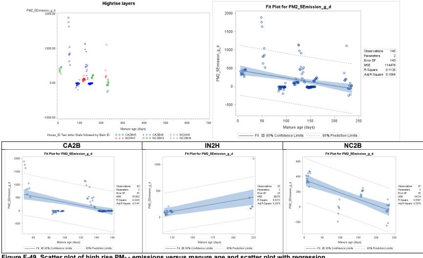
Figure F-49. Scatter plot of high rise PM<sub>2.5</sub> emissions versus manure age and scatter plot with regression.
