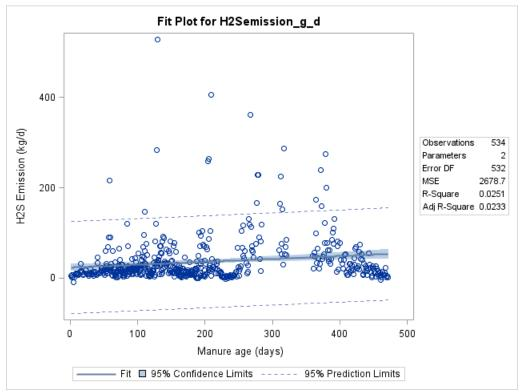
Figure F-161. Scatter plot of manure shed H₂S emissions versus manure age and scatter plot with regression.
