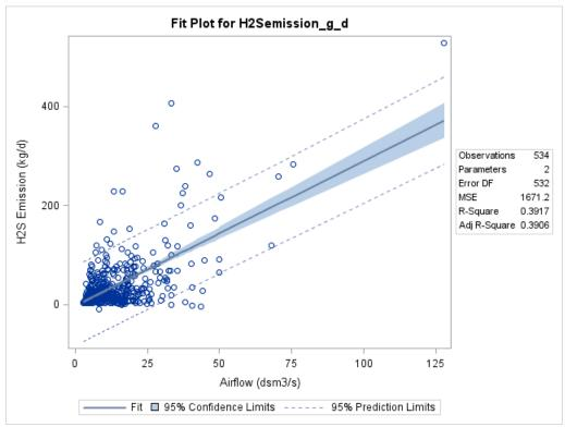
Figure F-141. Scatter plot of manure shed H₂S emissions versus airflow and scatter plot with regression.
