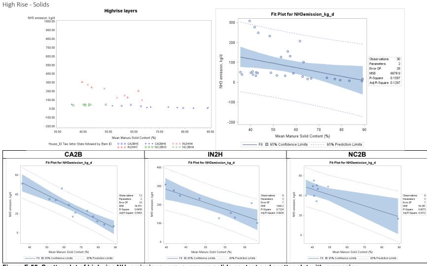
Figure F-55. Scatter plot of high rise NH<sub>3</sub> emissions versus manure solids content and scatter plot with regression.
