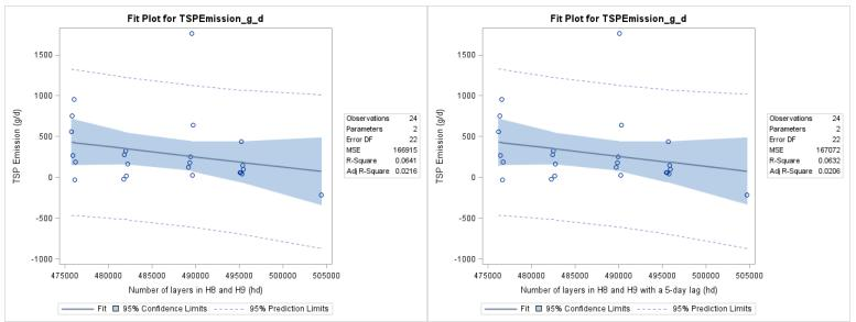
Figure F-124. Scatter plot, with regression of manure shed TSP emissions versus inventory (left) and inventory lagged by 5 days (right).
