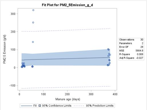
Figure F-163. Scatter plot of manure shed PM<sub>2.5</sub> emissions versus manure age and scatter plot with regression.
