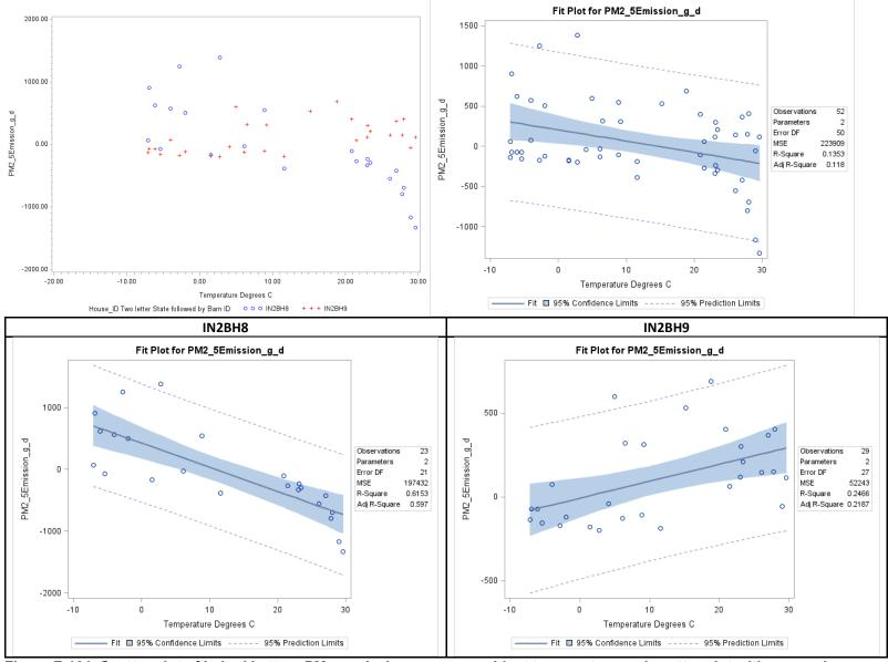
Figure F-101. Scatter plot of belted battery PM<sub>2.5</sub> emissions versus ambient temperature and scatter plot with regression.
