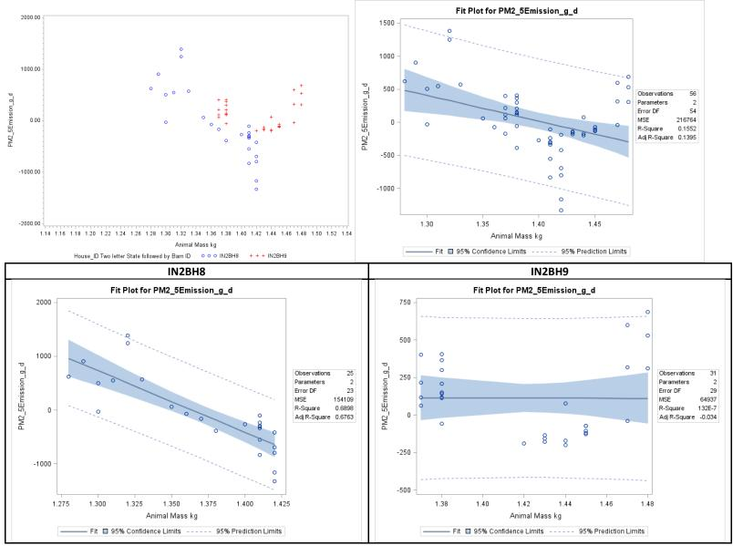
Figure F-71. Scatter plot of belted battery PM<sub>2.5</sub> emissions versus hen weight and scatter plot with regression.
