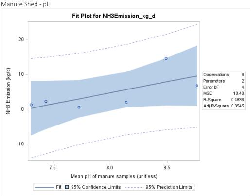
Figure F-165. Scatter plot of manure shed NH<sub>3</sub> emissions versus manure pH and scatter plot with regression.
