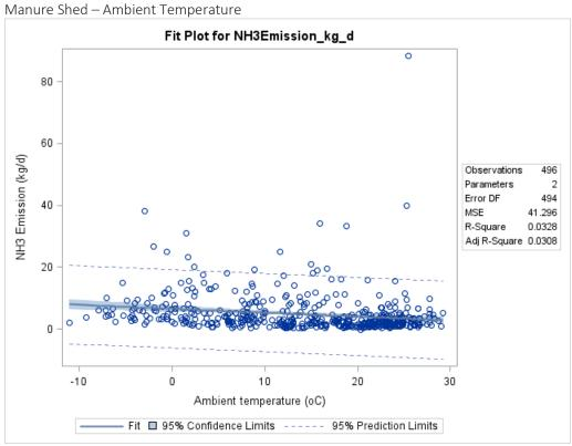
Figure F-145. Scatter plot of manure shed  $NH_3$  emissions versus ambient temperature and scatter plot with regression.
