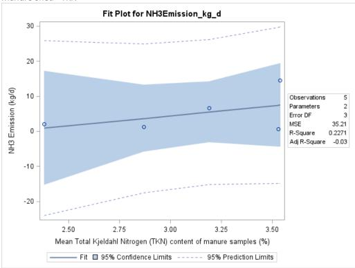
Figure F-174. Scatter plot of manure shed NH<sub>3</sub> emissions versus TKN and scatter plot with regression.
