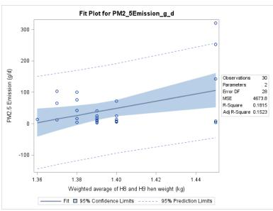
Figure F-128. Scatter plot of manure shed PM<sub>2.5</sub> emissions versus hen weight and scatter plot with regression.
