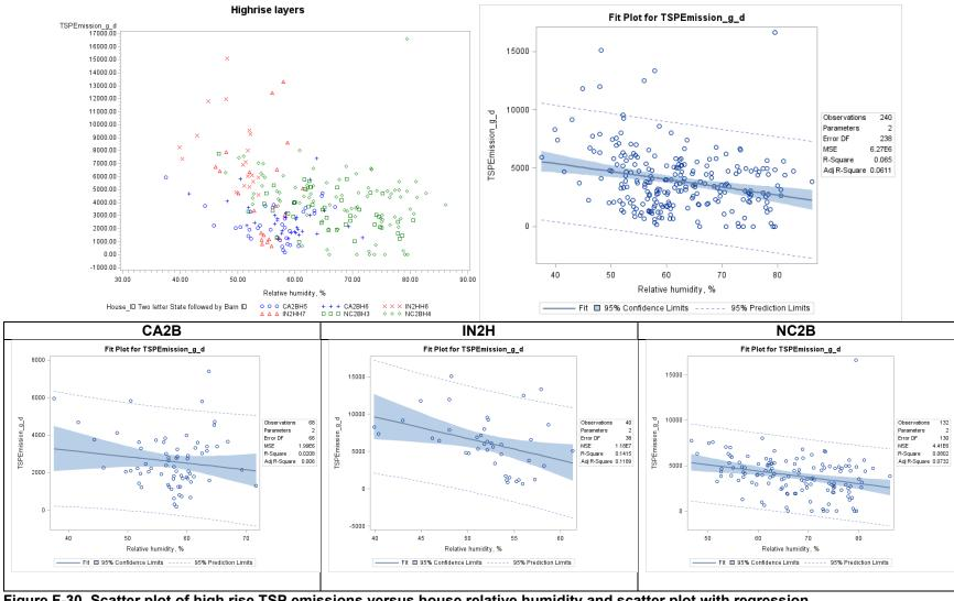
Figure F-30. Scatter plot of high rise TSP emissions versus house relative humidity and scatter plot with regression.
