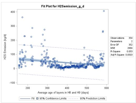
Figure F-136. Scatter plot of manure shed H<sub>2</sub>S emissions versus hen age and scatter plot with regression.
