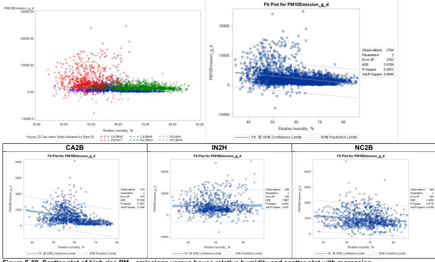
Figure F-28. Scatter plot of high rise PM<sub>10</sub> emissions versus house relative humidity and scatter plot with regression.
