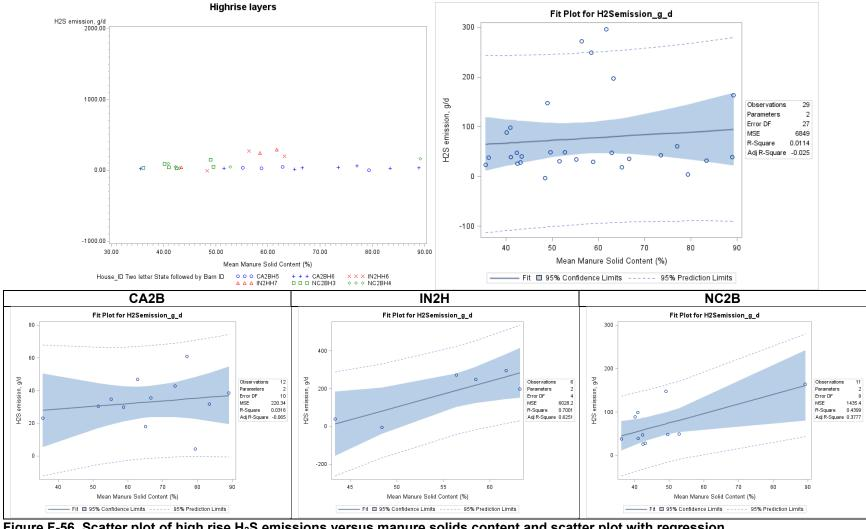
Figure F-56. Scatter plot of high rise H<sub>2</sub>S emissions versus manure solids content and scatter plot with regression.
