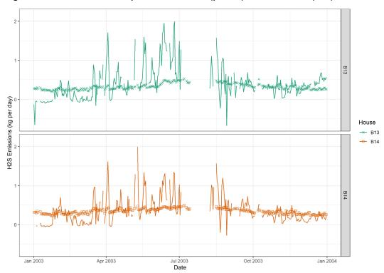
Figure H-2. Time series comparison of model (points) and observed (line) H<sub>2</sub>S emissions.
