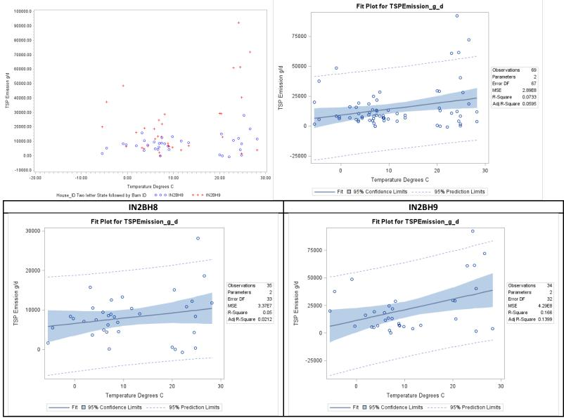
Figure F-102. Scatter plot of belted battery TSP emissions versus ambient temperature and scatter plot with regression.
