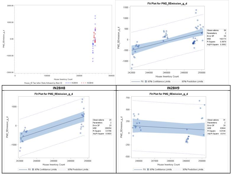
Figure F-66. Scatter plot of belted battery PM<sub>2.5</sub> emissions versus inventory and scatter plot with regression.
