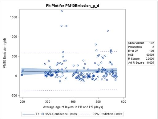
Figure F-137. Scatter plot of manure shed PM<sub>10</sub> emissions versus hen age and scatter plot with regression.
