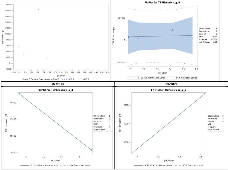
Figure F-111. Scatter plot of belted battery TSP emissions versus manure pH and scatter plot with regression.
