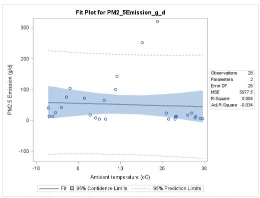
Figure F-148. Scatter plot of manure shed  $PM_{2.5}$  emissions versus ambient temperature and scatter plot with regression.
