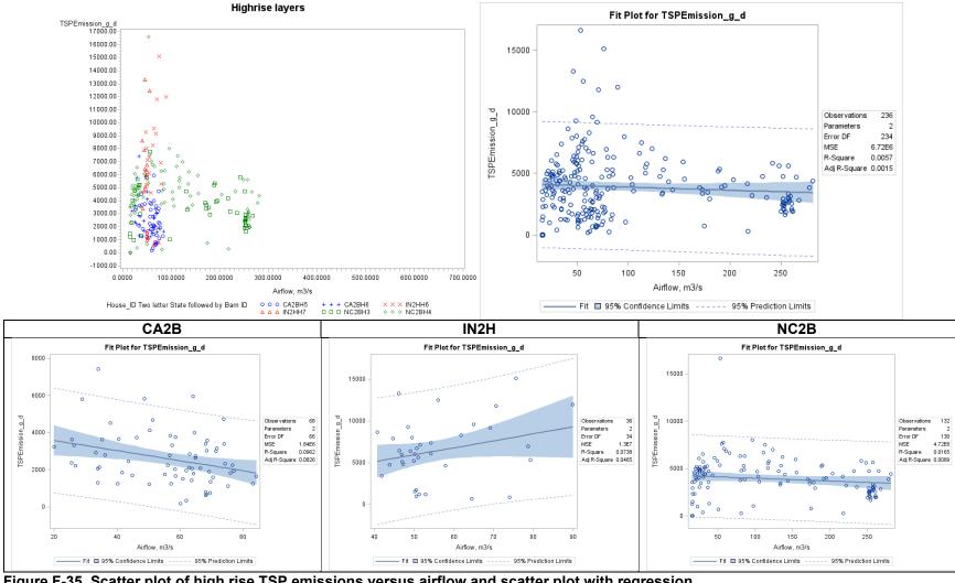
Figure F-35. Scatter plot of high rise TSP emissions versus airflow and scatter plot with regression.
