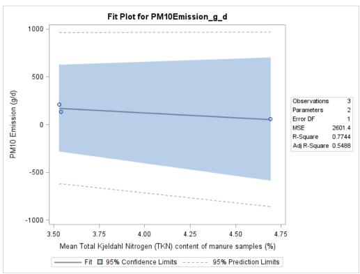
Figure F-176. Scatter plot of manure shed PM<sub>10</sub> emissions versus TKN and scatter plot with regression.
