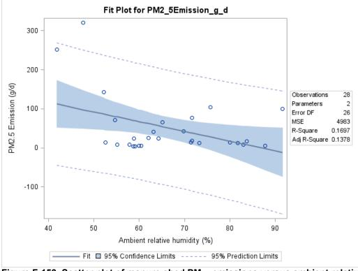
Figure F-153. Scatter plot of manure shed  $PM_{2.5}$  emissions versus ambient relative humidity and scatter plot with regression.
