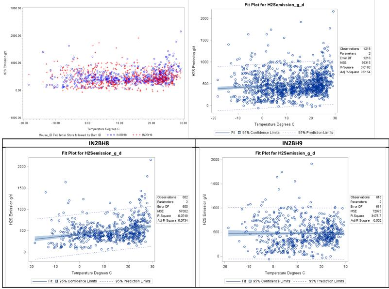
Figure F-99. Scatter plot of belted battery H<sub>2</sub>S emissions versus ambient temperature and scatter plot with regression.
