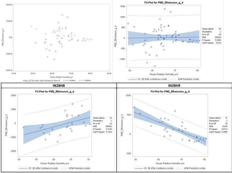
Figure F-91. Scatter plot of belted battery PM<sub>2.5</sub> emissions versus house relative humidity and scatter plot with regression.
