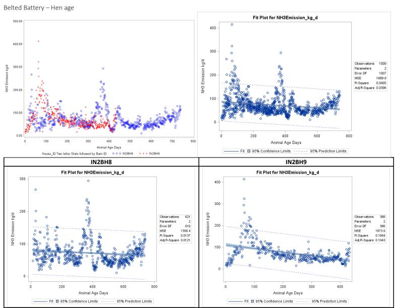
Figure F-78. Scatter plot of belted battery NH<sub>3</sub> emissions versus hen age and scatter plot with regression.
