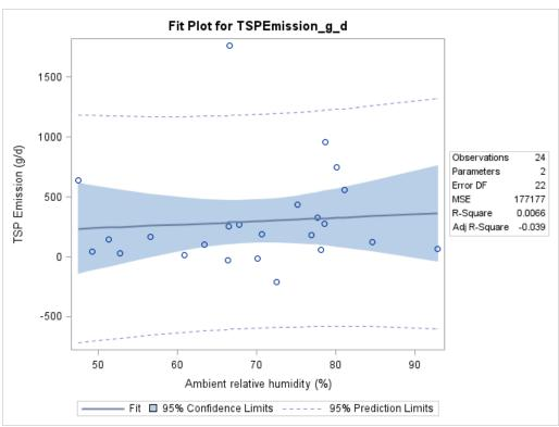
Figure F-154. Scatter plot of manure shed TSP emissions versus ambient relative humidity and scatter plot with regression.
