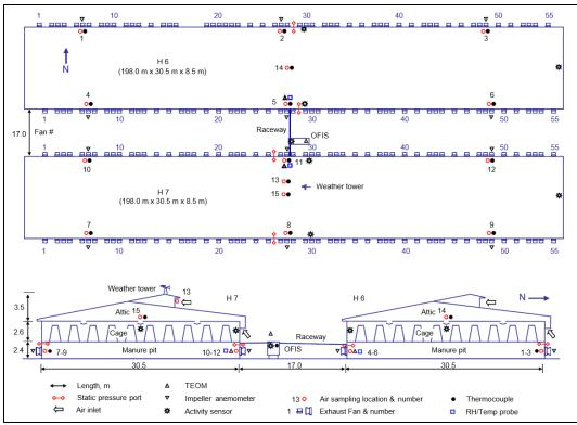
Figure 8-20. Overhead (top) and side (bottom) view of sensor measurements at IN2H (Ni et al. 2010a).
