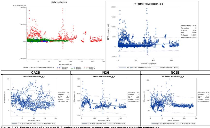
Figure F-47. Scatter plot of high rise H<sub>2</sub>S emissions versus manure age and scatter plot with regression.
