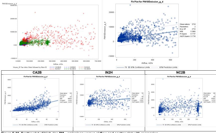
Figure F-33. Scatter plot of high rise PM<sub>10</sub> emissions versus airflow and scatter plot with regression.
