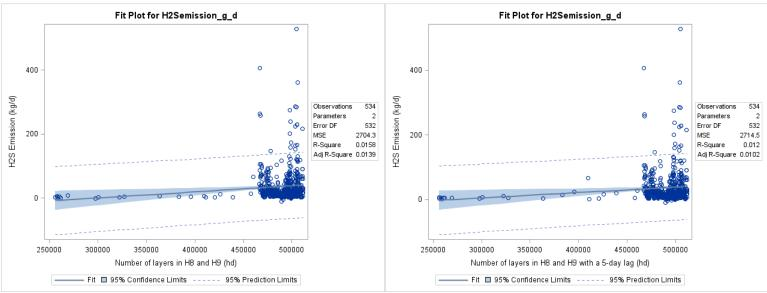
Figure F-121. Scatter plot, with regression of manure shed H<sub>2</sub>S emissions versus inventory (left) and inventory lagged by 5 days (right).
