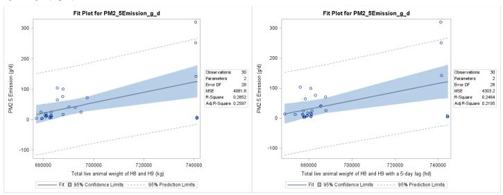
Figure F-133. Scatter plot, with regression of manure shed PM<sub>2.5</sub> emissions versus live animal weight (left) and live animal weight lagged by 5 days (right).
