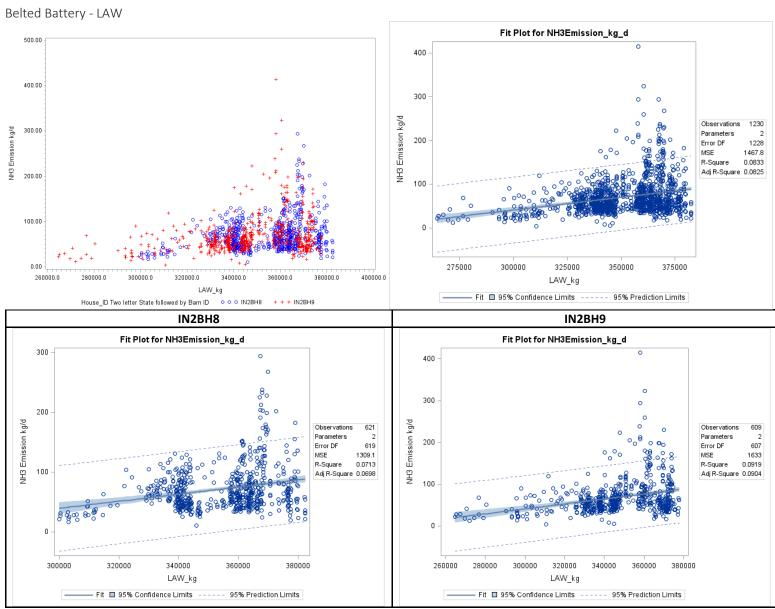
Figure F-73. Scatter plot of belted battery NH<sub>3</sub> emissions versus live animal weight and scatter plot with regression.
