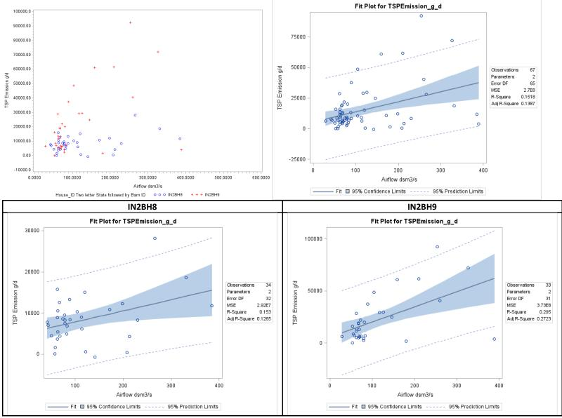
Figure F-97. Scatter plot of belted battery TSP emissions versus airflow and scatter plot with regression.
