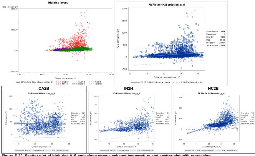
Figure F-22. Scatter plot of high rise H<sub>2</sub>S emissions versus exhaust temperature and scatter plot with regression.
