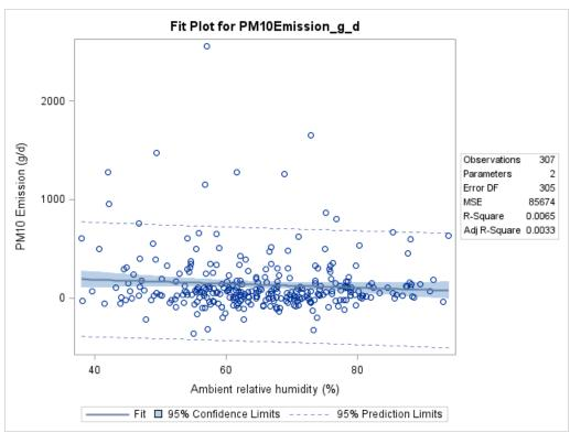
Figure F-152. Scatter plot of manure shed  $PM_{10}$  emissions versus ambient relative humidity and scatter plot with regression.
