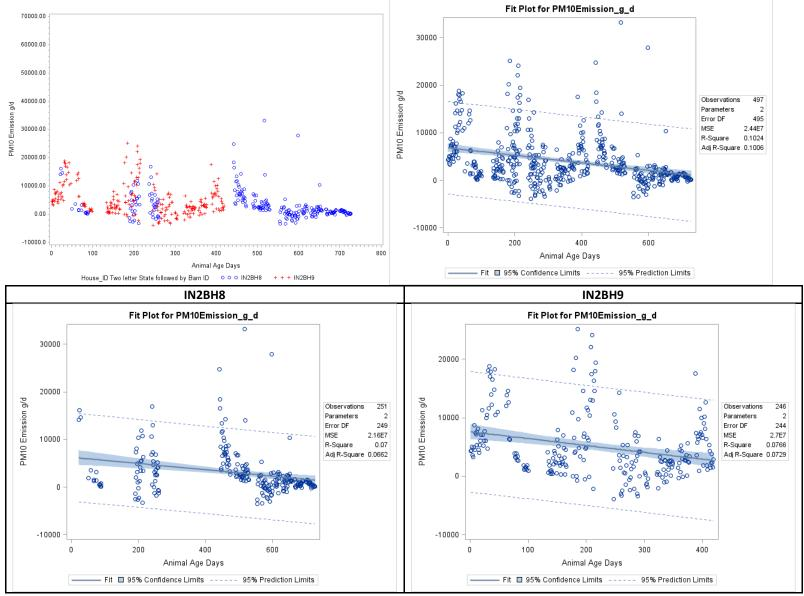
Figure F-80. Scatter plot of belted battery PM<sub>10</sub> emissions versus hen age and scatter plot with regression.
