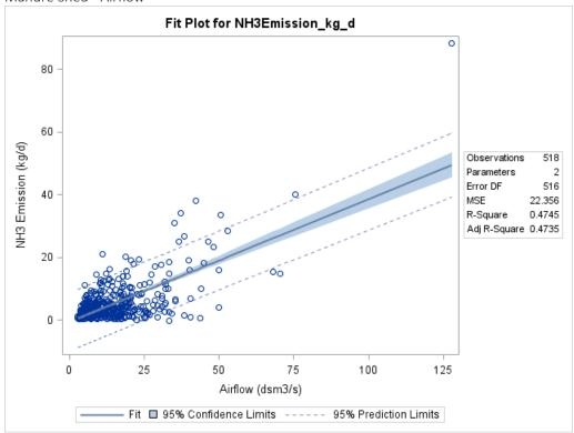
Figure F-140. Scatter plot of manure shed NH<sub>3</sub> emissions versus airflow and scatter plot with regression.
