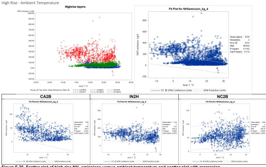
Figure F-36. Scatter plot of high rise NH<sub>3</sub> emissions versus ambient temperature and scatter plot with regression.
