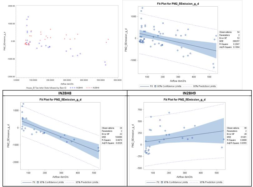
Figure F-96. Scatter plot of belted battery PM<sub>2.5</sub> emissions versus airflow and scatter plot with regression.
