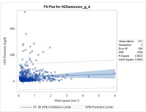
Figure F-156. Scatter plot of manure shed H₂S emissions versus wind speed and scatter plot with regression.
