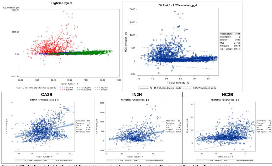
Figure F-27. Scatter plot of high rise H<sub>2</sub>S emissions versus house relative humidity and scatter plot with regression.
