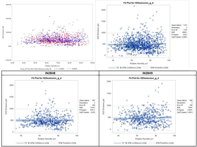
Figure F-104. Scatter plot of belted battery H₂S emissions versus ambient relative humidity and scatter plot with regression.
