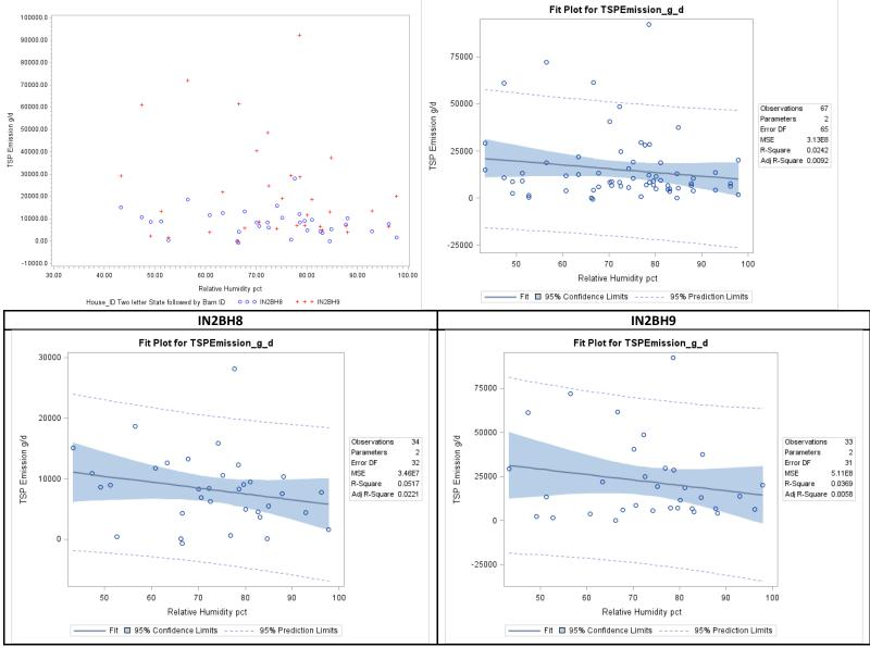
Figure F-107. Scatter plot of belted battery TSP emissions versus ambient relative humidity and scatter plot with regression.
