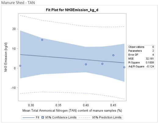
Figure F-171. Scatter plot of manure shed  $NH_3$  emissions versus TAN and scatter plot with regression.
