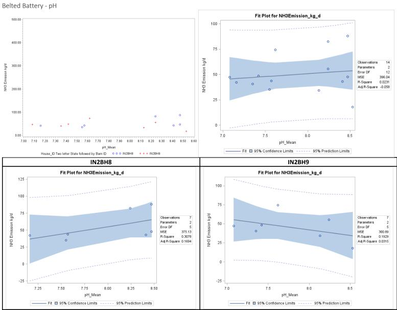
Figure F-108. Scatter plot of belted battery NH<sub>3</sub> emissions versus manure pH and scatter plot with regression.
