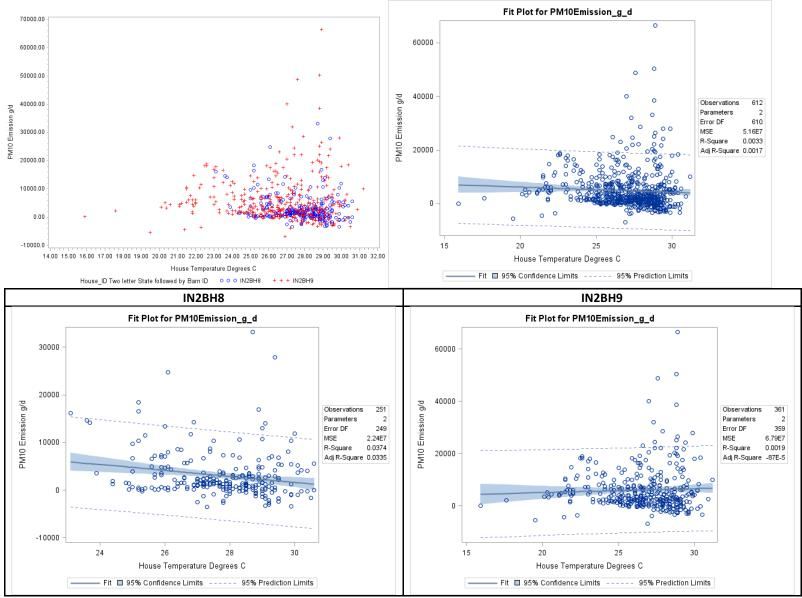
Figure F-85. Scatter plot of belted battery PM<sub>10</sub> emissions versus exhaust temperature and scatter plot with regression.
