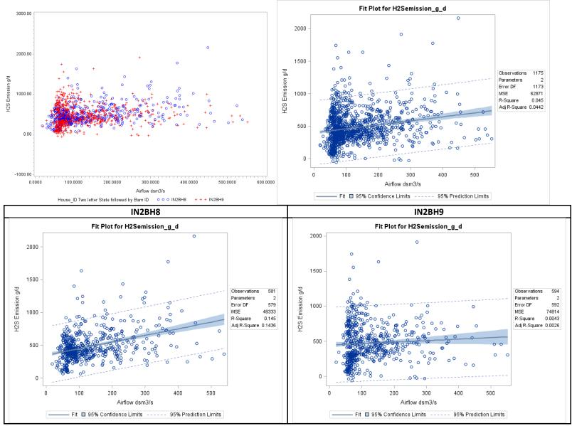
Figure F-94. Scatter plot of belted battery H₂S emissions versus airflow and scatter plot with regression.
