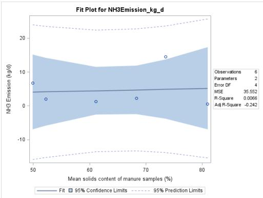
Figure F-168. Scatter plot of manure shed NH<sub>3</sub> emissions versus manure solids content and scatter plot with regression.
