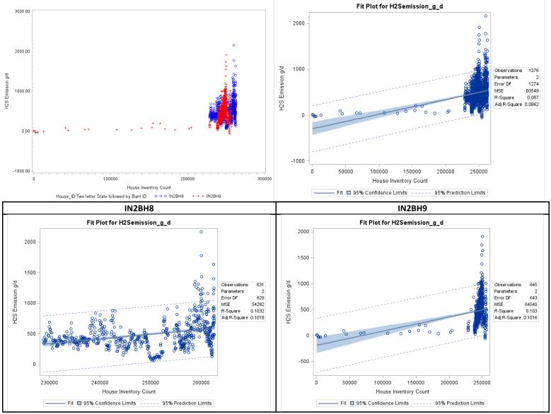
Figure F-64. Scatter plot of belted battery H<sub>2</sub>S emissions versus inventory and scatter plot with regression.
