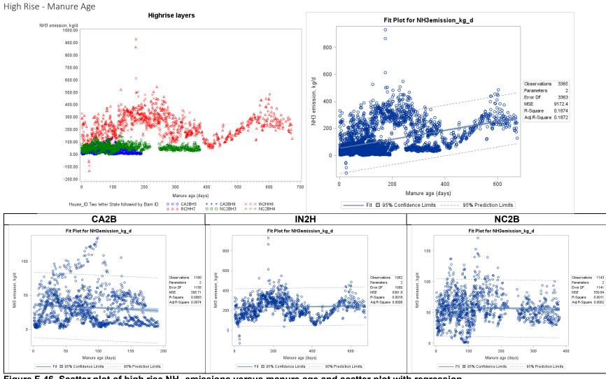
Figure F-46. Scatter plot of high rise NH<sub>3</sub> emissions versus manure age and scatter plot with regression.
