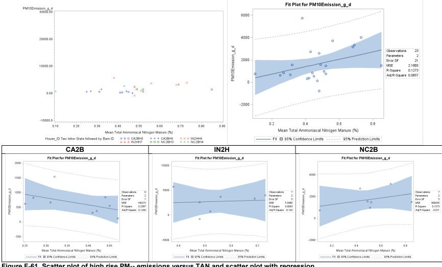
Figure F-61. Scatter plot of high rise PM<sub>10</sub> emissions versus TAN and scatter plot with regression.
