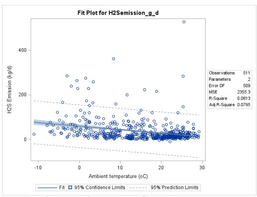
Figure F-146. Scatter plot of manure shed H₂S emissions versus ambient temperature and scatter plot with regression.
