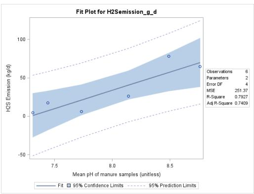
Figure F-166. Scatter plot of manure shed H₂S emissions versus manure pH and scatter plot with regression.
