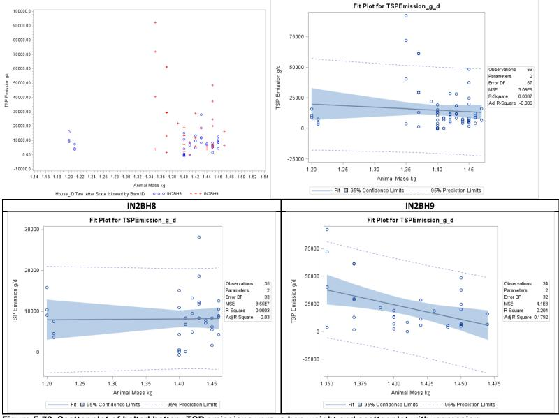
Figure F-72. Scatter plot of belted battery TSP emissions versus hen weight and scatter plot with regression.
