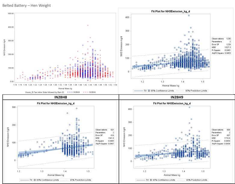
Figure F-68. Scatter plot of belted battery NH<sub>3</sub> emissions versus hen weight and scatter plot with regression.
