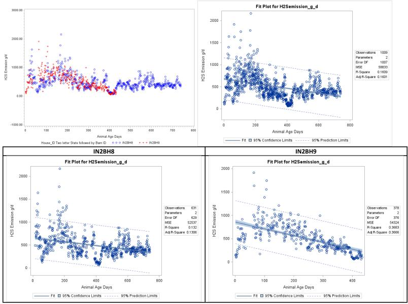
Figure F-79. Scatter plot of belted battery H<sub>2</sub>S emissions versus hen age and scatter plot with regression.
