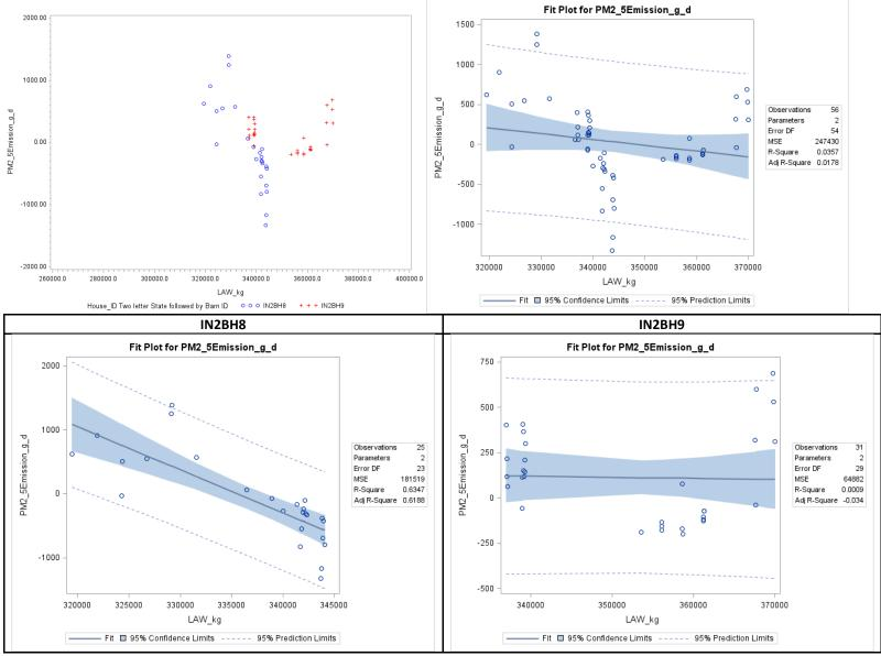
Figure F-76. Scatter plot of belted battery PM<sub>2.5</sub> emissions versus live animal weight and scatter plot with regression.
