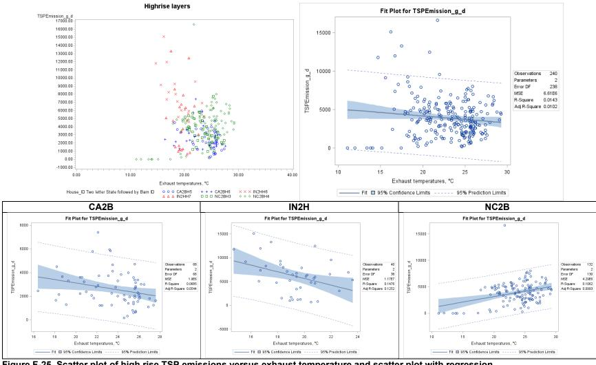
Figure F-25. Scatter plot of high rise TSP emissions versus exhaust temperature and scatter plot with regression.
