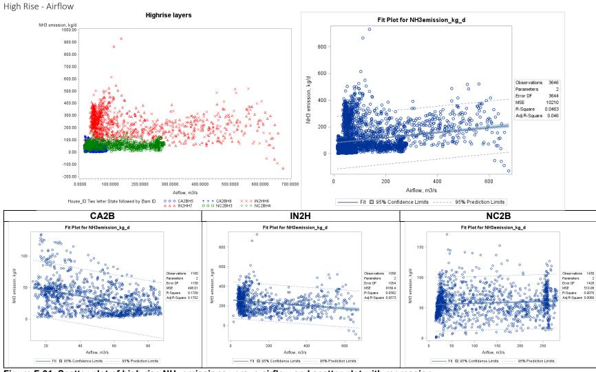
Figure F-31. Scatter plot of high rise NH<sub>3</sub> emissions versus airflow and scatter plot with regression.
