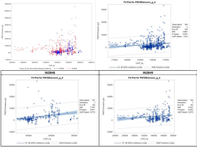
Figure F-75. Scatter plot of belted battery PM<sub>10</sub> emissions versus live animal weight and scatter plot with regression.
