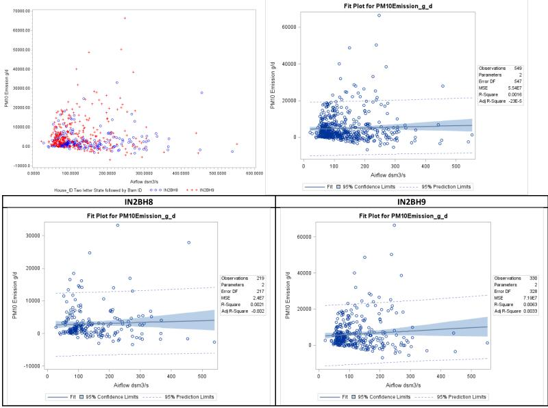
Figure F-95. Scatter plot of belted battery PM<sub>10</sub> emissions versus airflow and scatter plot with regression.
