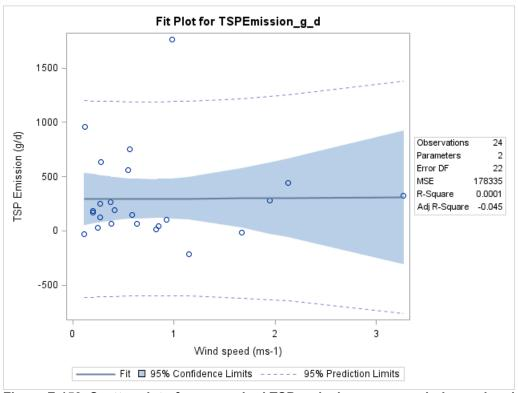
Figure F-159. Scatter plot of manure shed TSP emissions versus wind speed and scatter plot with regression.
