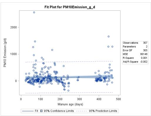
Figure F-162. Scatter plot of manure shed PM<sub>10</sub> emissions versus manure age and scatter plot with regression.
