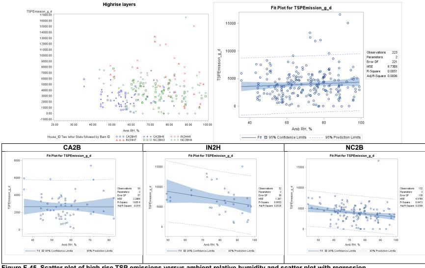
Figure F-45. Scatter plot of high rise TSP emissions versus ambient relative humidity and scatter plot with regression.
