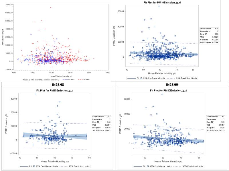
Figure F-90. Scatter plot of belted battery PM<sub>10</sub> emissions versus house relative humidity and scatter plot with regression.
