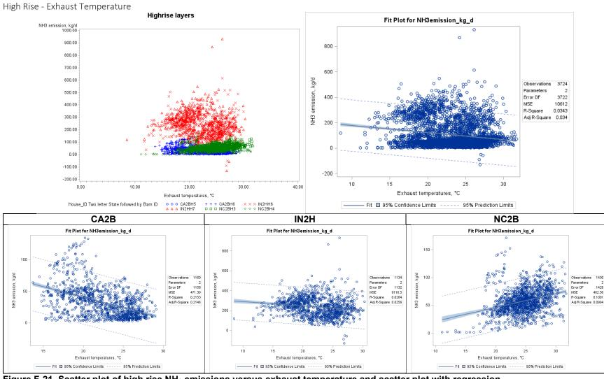
Figure F-21. Scatter plot of high rise NH<sub>3</sub> emissions versus exhaust temperature and scatter plot with regression.
