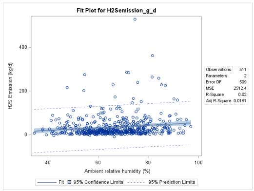
Figure F-151. Scatter plot of manure shed  $H_2S$  emissions versus ambient relative humidity and scatter plot with regression.
