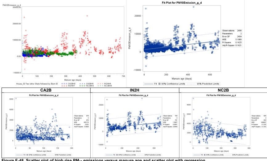
Figure F-48. Scatter plot of high rise PM<sub>10</sub> emissions versus manure age and scatter plot with regression.
