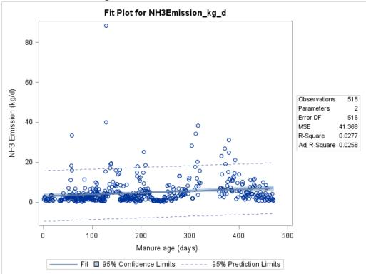
Figure F-160. Scatter plot of manure shed NH<sub>3</sub> emissions versus manure age and scatter plot with regression.
