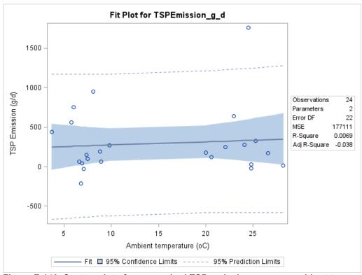
Figure F-149. Scatter plot of manure shed TSP emissions versus ambient temperature and scatter plot with regression.
