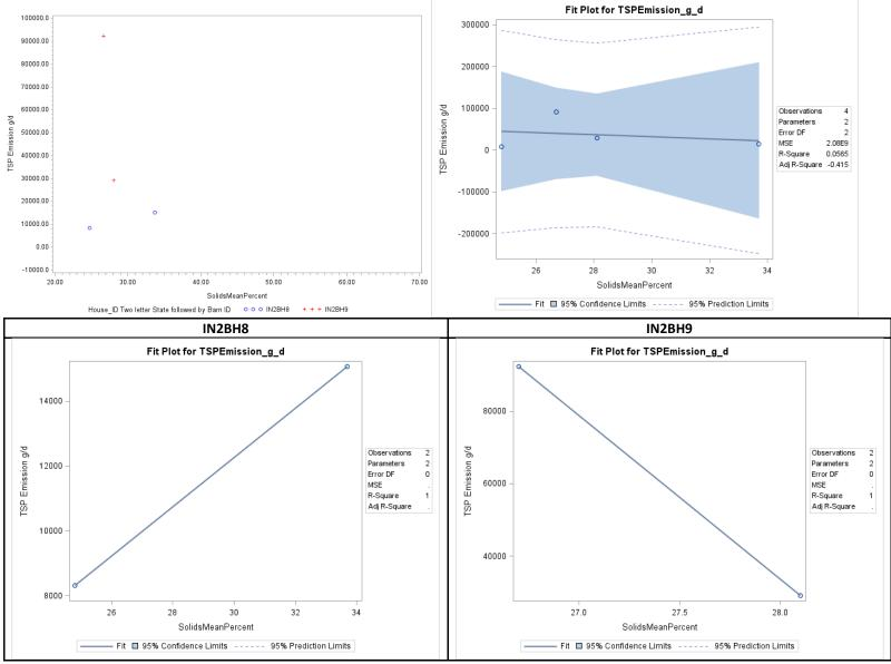
Figure F-115. Scatter plot of belted battery TSP emissions versus manure solids content and scatter plot with regression.
