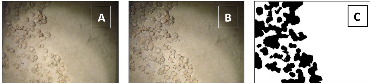
Figure 6. Dreissena in original clipped still image before highlighting (A) with Dreissena highlighted (B) and in black and white image after highlighting (C). In highlighted images Dreissena appear black and the background appears white. Dreissena coverage (%) is calculated by dividing the area covered by mussels (black) by total area of the image.
