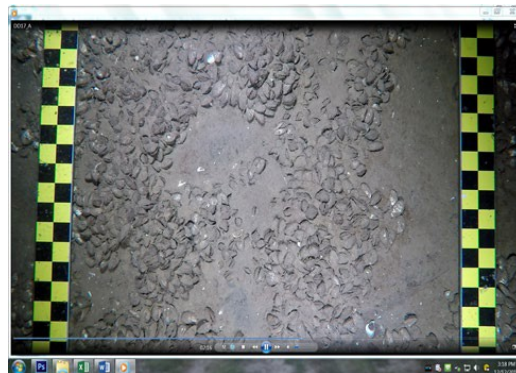
Figure 2. Black or yellow squares on the scale bar of the drop-down camera frame will be used to set the measurement scale in Photoshop.
