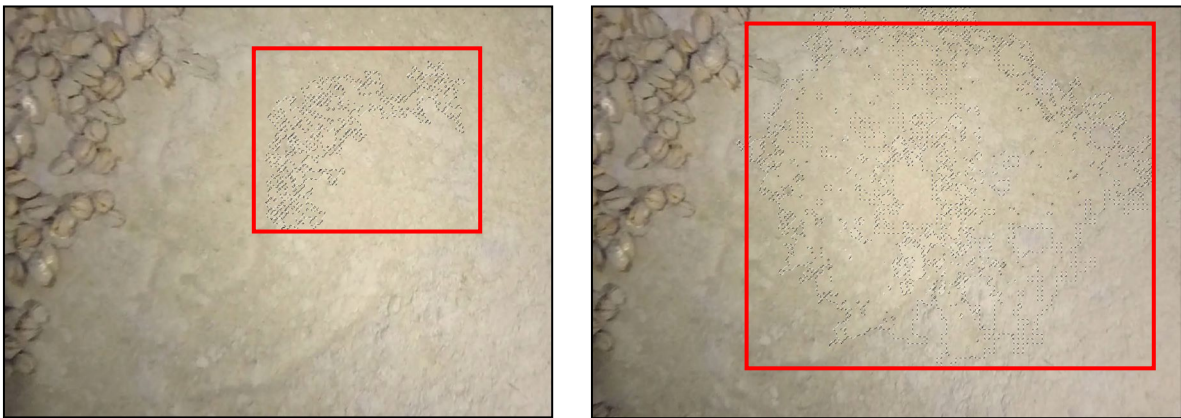
Figure 4. Area selected in still image by using Point Sample (left) vs. area selected by using a Sample Size of 3x3 pixels (right).
