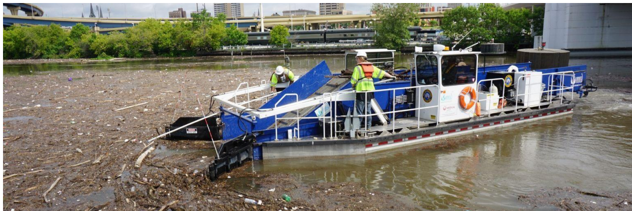
Figure 13. Milwaukee Metropolitan Sewerage District’s river skimmer (Lynyrd Skymmr) cleaning up garbage and floating debris in the Menomonee River near the N 6 th Street bridge (Vitran, 2019).
