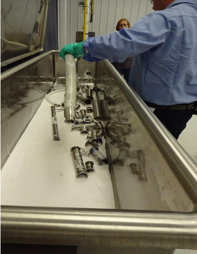
Figure 5. Subject removing sanitized equipment/parts from COP tank.
