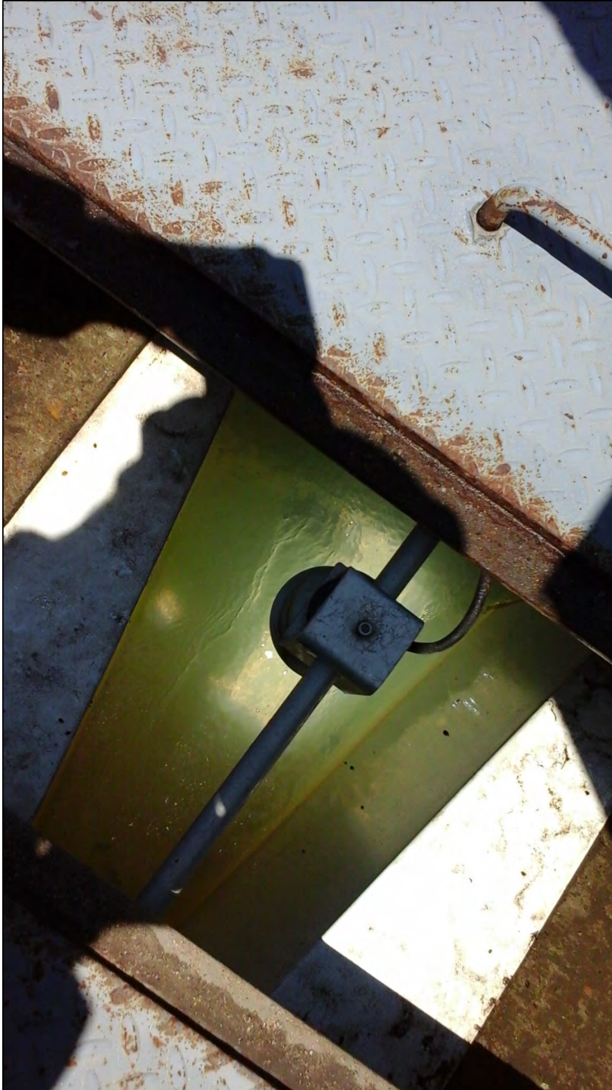
Photograph 15. Additional view of the turbulence observed in the Outfall 003B Parshall flume.
