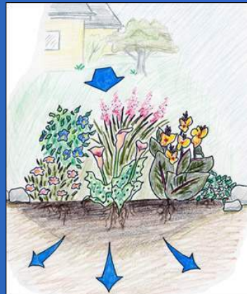
Water enters the rain garden, then dissipates slowly into the ground
