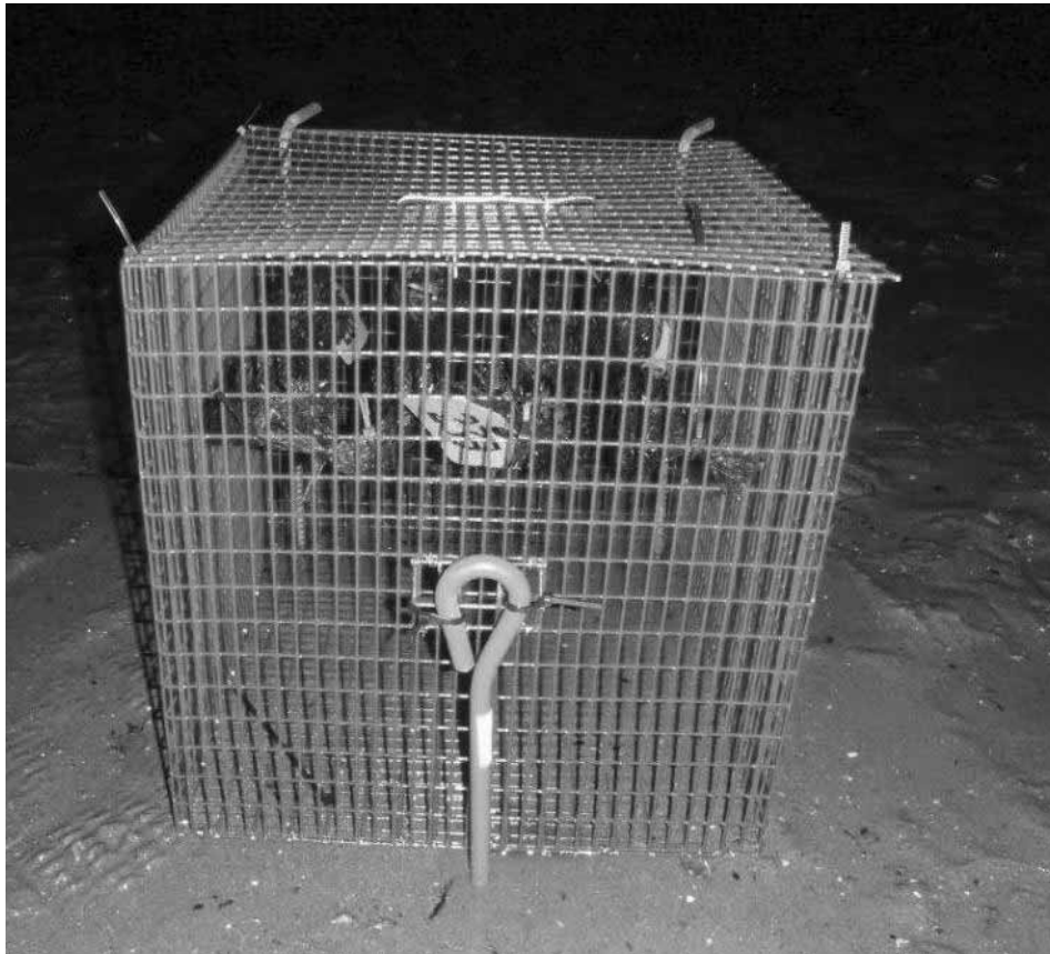
Figure 8. Mussel monitoring cage driven through with bent-tip rebar stakes (on the far end) and secured to a helical anchor with cable ties. For better cage anchoring, 3-4 rebar stakes are recommended.
