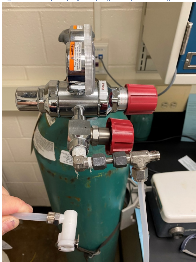
Figure 6: Example of N_2 tank, regulator, and tubing.
