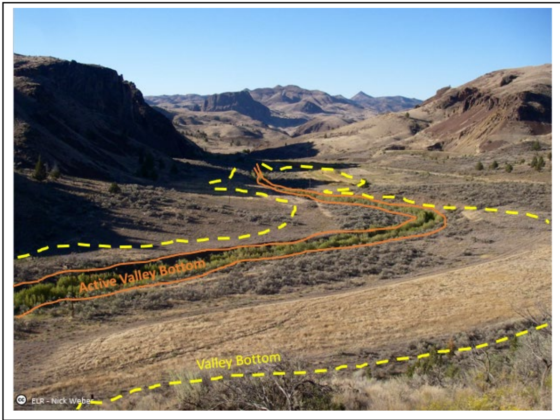
Figure 10. Example of Active Valley Bottom Width Compared to Valley Bottom Width.
