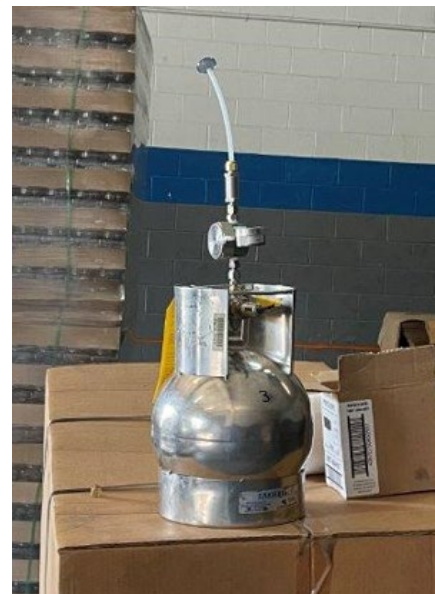
Figure 2 Summa Cannister for Indoor Air Sampling
