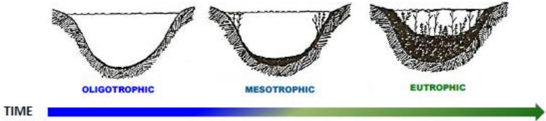
Figure 2-1. Conceptual diagram depicting the process of eutrophication in lakes. Eutrophication is the natural process by which nutrients, organic matter, and sediments gradually accumulate within a waterbody, resulting in decreased depth and increased biological productivity.
