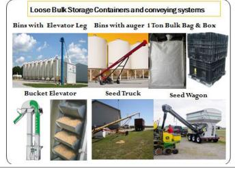
Downstream facilities process much of their seed as loose bulk, where treated seed is conveyed into a grower's truck or wagon directly from the treater. This is distinctly different from on-farm seed treating where seed is treated more locally (e.g., at a specific farm), and planted without bagging. All on-farm seed treatment systems have a method to transfer and treat clean untreated seed from bulk storage to a seed wagon or truck, or from a truck or wagon to the planter.
