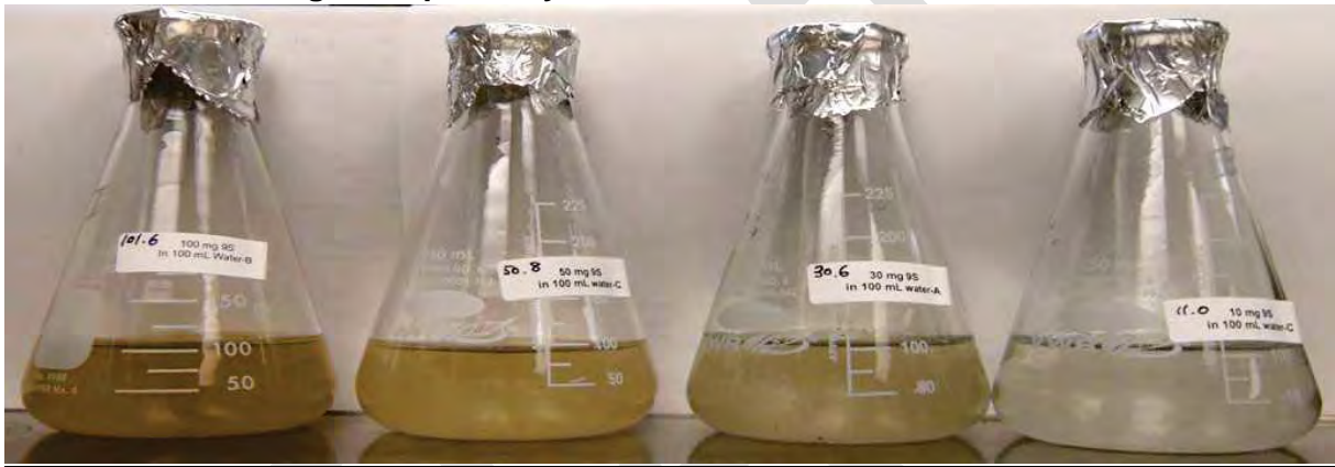
Figure 4. Appearance of a 100 mL aqueous sample containing 100, 50, 30 and 10 mg of solids from left to right, respectively.
