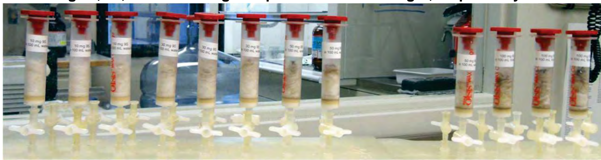
Figure 6. Appearance of 150 mg WAX SPE cartridges packed with glass wool to half the height of the cartridge barrel. Picture taken after passing aqueous samples containing 10, 30, 50 and 100 mg in triplicate from left to right, respectively.
