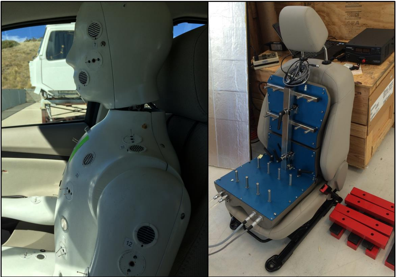
Figure 6. HVAC (left) and STAN (right) testing manikins used for experimental testing
