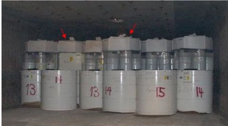
Figure 4-5. MgO supersacks placed on waste canisters. Red arrows showing the MgO supersacks placed on waste canisters. Adapted from Figure 1 of Appendix MgO (DOE 2014a)
